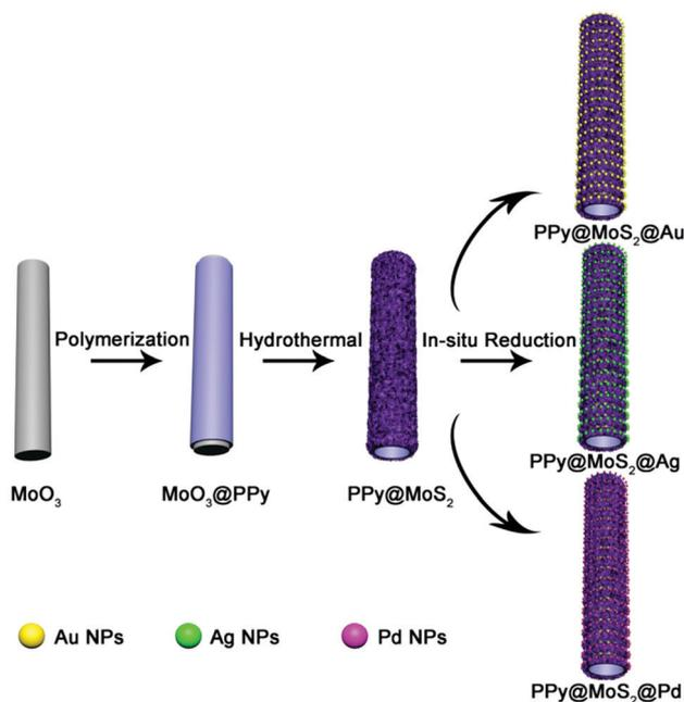
Scheme 1 Schematic synthesis of PPy@MoS<sub>2</sub>@Au/Ag/Pd composites.
