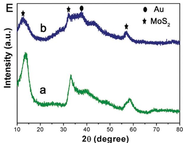
Fig. 2 SEM and TEM images of PPy@MoS<sub>2</sub> (A and B) and PPy@MoS<sub>2</sub>@Au (C and D) and (E) XRD patterns of PPy@MoS<sub>2</sub> (a) and PPy@MoS<sub>2</sub>@Au (b). Scale bars: 1  $\mu\text{m}$  in (A) and 500 nm in (B–D).
