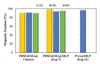
Fig. 8 Magnetic fraction ( $\omega_{mag}$ ) obtained at different times of magnetic separation for the PDMAEMA@clusters, and the PDMAEMA@MLP (Exp. 7) and PAA@MLP (Exp. 11) samples obtained by seeded emulsion polymerization of styrene (Tables 1 and 2).
