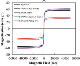
Fig. 7 (A) TGA and (B) SQUID analyses of the commercial fatty acidmodified IO nanoparticles (FA@IONPs), the PDMAEMA@clusters, the PAA@clusters, and the magnetic fraction ( $\omega_{mag}$ ) of the PDMAEMA@MLP and PAA@MLP samples (Exp. 7, Table 1 and Exp. 11, Table 2).
