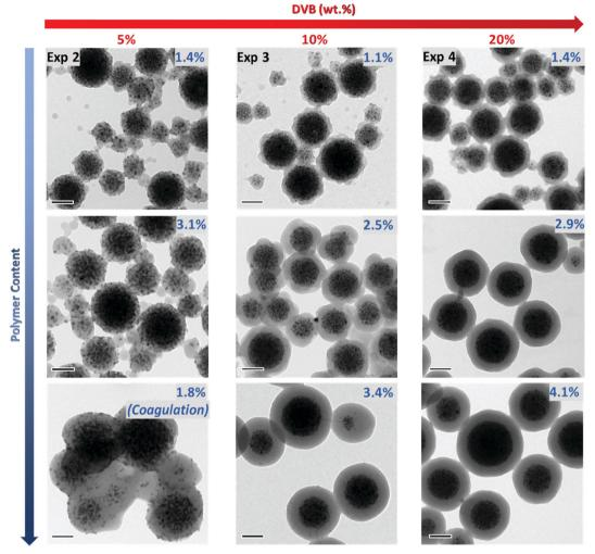
Fig. 3 TEM micrographs of PDMAEMA@MLPs ( $PC_{theo} = 10\%$ ) synthesized in the presence of increasing amounts of DVB (based on overall monomer mass): 5 wt%, 10 wt% and 20 wt% (Exp. 2, 3 and 4, respectively, Table 1). The images from top to bottom correspond to samples taken at different reaction times and therefore, to increasing polymer contents. Scale bar: 100 nm.
