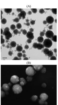
Fig. 6 (A) TEM and (B) SEM micrographs of PAA@MLPs synthesized by seeded semi-batch emulsion polymerization of styrene with 23 wt% DVB (Exp. 11, Table 2). Scale bar = 100 nm
