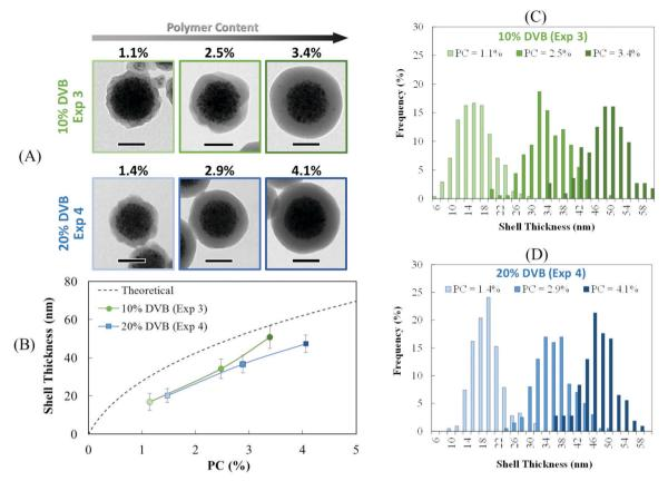
Fig. 4 Evolution of the shell thickness with the polymer content for PDMAEMA@MLPs prepared by seeded emulsion polymerization of styrene in the presence of 10 and 20 wt% of DVB (Exp. 3 and 4, respectively, Table 1). The theoretical shell thickness was calculated according to egn (5) and (6).
