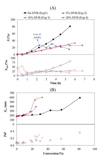
Fig. 2 Effect of DVB content on (A) the instantaneous ( $X_{inst}$ , empty symbols) and global conversions (X, filled symbols) with time and (B) the particle size ( $Z_{av}$ , filled symbols) and size dispersity (PdI, empty symbols) with conversion, for the seeded semi-batch emulsion polymerization of styrene using PDMAEMA@clusters as seeds. The theoretical polymer and IO contents were fixed at around 12 and 11 wt%, respectively (Exp. 1-4, Table 1)
