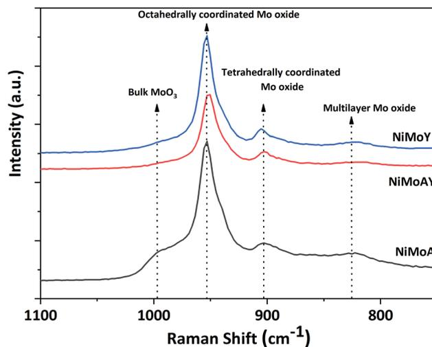
Fig. 7 Raman spectra of the synthesized catalyst.
