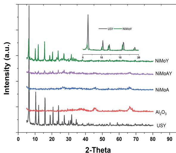
Fig. 6 XRD pattern of the synthesized catalysts, parent USY and  $\gamma$ -Al<sub>2</sub>O<sub>3</sub>.
