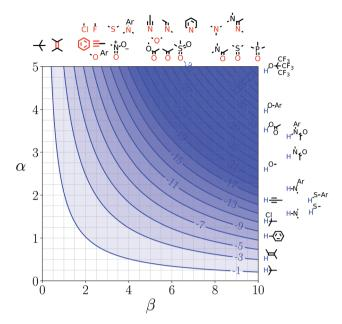
Fig. 3 FGIP for the interaction of two solutes in a hypothetical room temperature liquid state of a noble gas where the concentration of solvent SSIPs is 160 M ( $\Delta\Delta G_{\rm FGI}$  in kJ mol<sup>-1</sup>).
