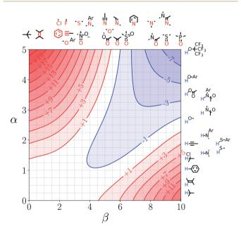
Fig. 5 FGIP for the interaction of two solutes in ethanol at 298 K  $(\Delta\Delta G_{\text{FGI}} \text{ in kJ mol}^{-1})$ . The solute-solute interactions are favourable in the blue region, and unfavourable in the red region.
