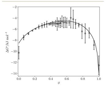
Fig. 12  $\Delta G^{\circ}$  (kJ mol<sup>-1</sup>) for formation of a 1 : 1 complex between tri-n-butylphosphine oxide ( $\beta=10.7$ ) and 4-phenyl azophenol ( $\alpha=4.1$ ) in THF-chloroform mixtures. Experimental measurements (black circles) and calculated values using eqn (16) (black line) as function of chloroform volume fraction,  $\phi$ . The experimental values are the average of five experiments with error bars at the 95% confidence limit.
