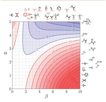
**Fig. 6** FGIP for the interaction of two solutes in 1,1,1,3,3,3-hexafluoro-2-propanol at 298 K ( $\Delta\Delta G_{\text{FGI}}$  in kJ  $\text{mol}^{-1}$ ). The solute–solute interactions in the blue region, and unfavourable in the red region.
