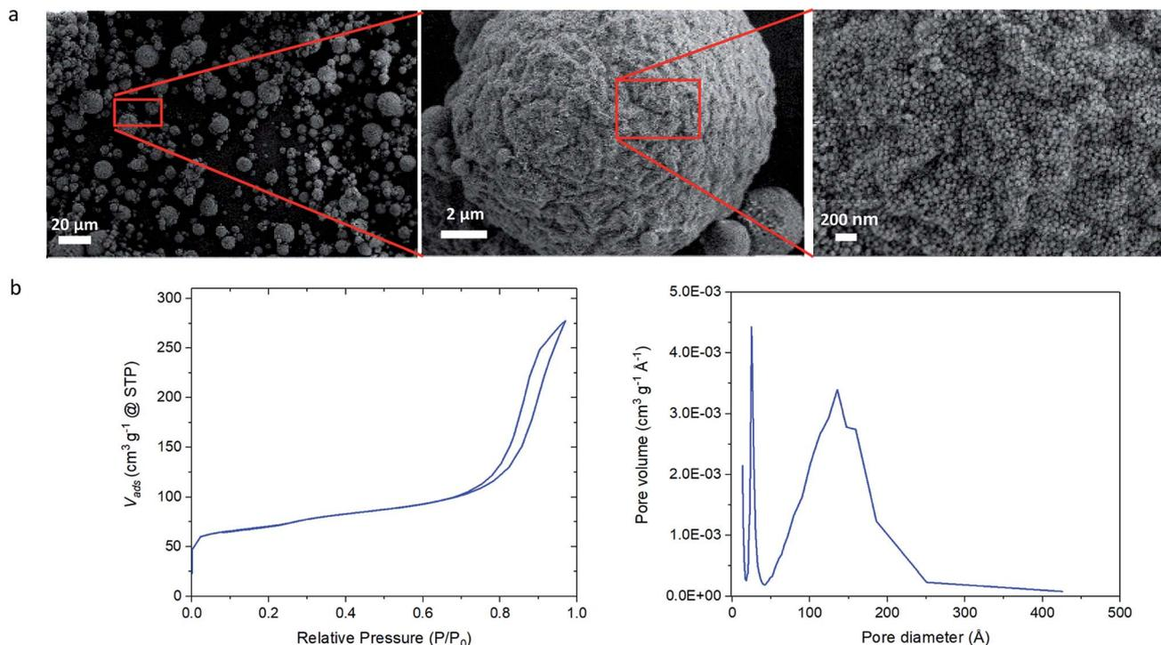
Fig. 3 Characterization of MZSM particles. (a) SEM images of the prepared MZSMs particles. (b) N<sub>2</sub> isotherm and N<sub>2</sub> adsorption pore size distribution of the MZSMs.
