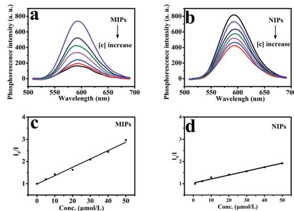
Fig. 10 (a) The RTP emission spectra of Mn-doped ZnS QD@ms-MIPs ( $30 \text{ mg L}^{-1}$ ) and (b) Mn-doped ZnS QD@ms-NIPs ( $30 \text{ mg L}^{-1}$ ) with the addition of different concentrations of phenol in DDW. The Stern–Volmer values for (c) Mn-doped ZnS QDs@ms-MIPs and (d) Mn-doped ZnS QDs@ms-NIPs.
