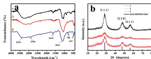
Fig. 3 (a) FT-IR spectra of MPTS-ZnS QDs:Mn (curve 1), Mn-doped ZnS QD@MIPs (curve 2) and Mn-doped ZnS QD@ms-MIPs (curve 3); (b) XRD patterns of MPTS-ZnS QDs:Mn (curve 1), Mn-doped ZnS QD@MIPs (curve 2) and Mn-doped ZnS QD@ms-MIPs (curve 3).
