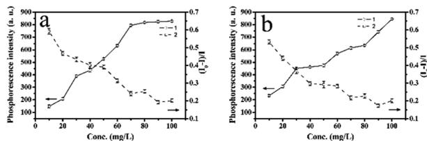
Fig. 7 (a) Effect of concentration of the Mn-doped ZnS QD@MIPs on the RTP intensity and by adding quantitative phenol ( $5 \text{ mg L}^{-1}$ , curve 1), the quenching efficiency for different concentrations of the Mn-doped ZnS QD@MIPs (curve 2); (b) effect of concentration of the Mn-doped ZnS QD@ms-MIPs on the RTP intensity and by adding quantitative phenol ( $5 \text{ mg L}^{-1}$ , curve 1), the quenching efficiency for different concentrations of the Mn-doped ZnS QD@ms-MIPs (curve 2).
