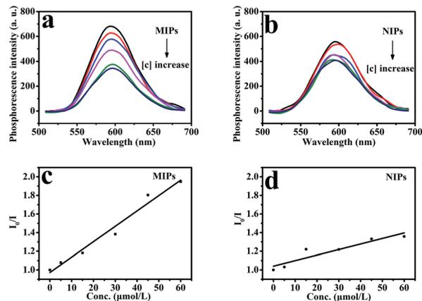
Fig. 9 (a) The RTP emission spectra of Mn-doped ZnS QD@MIPs ( $45 \text{ mg L}^{-1}$ ) and (b) Mn-doped ZnS QD@NIPs ( $45 \text{ mg L}^{-1}$ ) with addition of different concentrations of phenol in DDW. The Stern–Volmer values for (c) Mn-doped ZnS QDs@MIPs and (d) Mn-doped ZnS QDs@NIPs.
