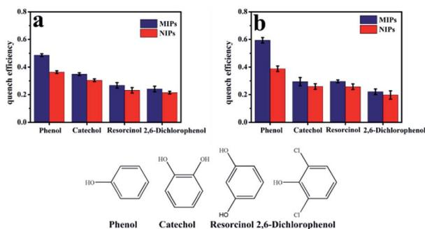
Fig. 11 (a) The selectivity of Mn-doped ZnS QD@mIPs and Mn-doped ZnS QD@ms-NIPs with the addition of several similar structural of phenols ( $5.0 \text{ mg L}^{-1}$ ); (b) the selectivity of Mn-doped ZnS QD@ms-MIPs and Mn-doped ZnS QD@ms-NIPs with the addition of several similar structural of phenols ( $5.0 \text{ mg L}^{-1}$ ).
