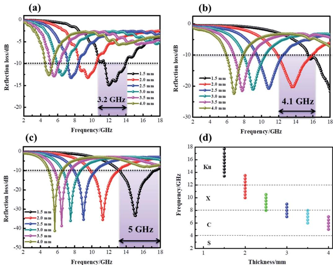
Fig. 9 Reflection loss curves of CF (a), CF@CoFe<sub>2</sub>O<sub>4</sub> (b) and CF@CoFe<sub>2</sub>O<sub>4</sub>@MnO<sub>2</sub> composite (c) at a different thickness, the effective absorption band width of CF@CoFe<sub>2</sub>O<sub>4</sub>@MnO<sub>2</sub> composite (d).
