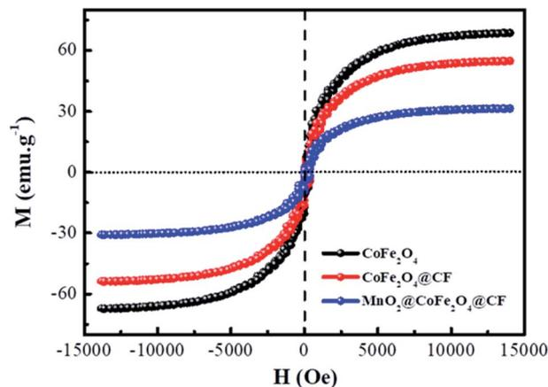
Fig. 6 Hysteresis loops of CoFe<sub>2</sub>O<sub>4</sub>, CF@CoFe<sub>2</sub>O<sub>4</sub> and CF@CoFe<sub>2</sub>O<sub>4</sub>@MnO<sub>2</sub> composites.
