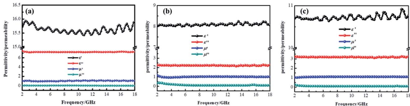
Fig. 7 Electromagnetic parameters of CF (a), CF@CoFe<sub>2</sub>O<sub>4</sub> (b) and CF@CoFe<sub>2</sub>O<sub>4</sub>@MnO<sub>2</sub> composite (c).
