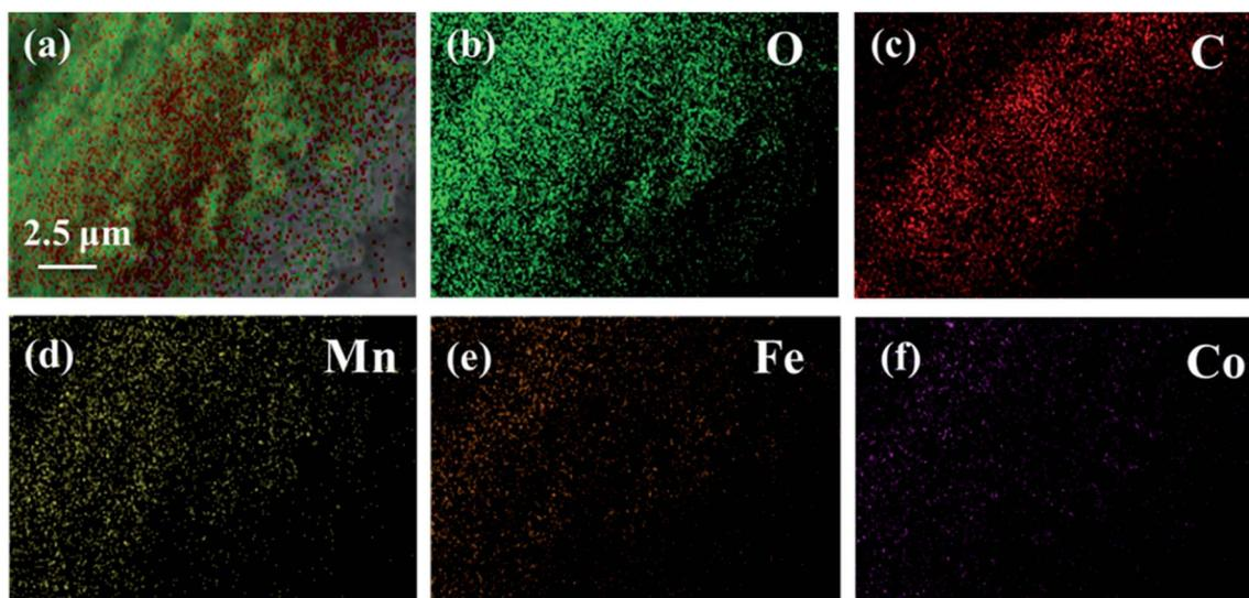
Fig. 3 EDX elemental mapping images (a–f) of CF@CoFe<sub>2</sub>O<sub>4</sub>@MnO<sub>2</sub> composite.
