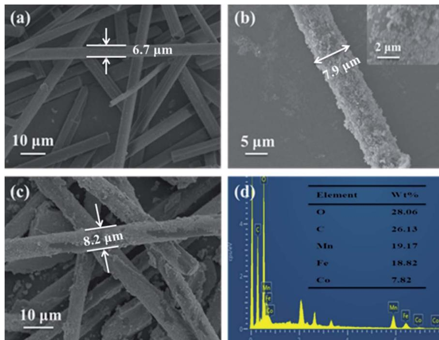
Fig. 2 SEM images of CF (a), CF@CoFe<sub>2</sub>O<sub>4</sub> (b), CF@CoFe<sub>2</sub>O<sub>4</sub>@MnO<sub>2</sub> composites (c) and the EDS spectra of CF@CoFe<sub>2</sub>O<sub>4</sub>@MnO<sub>2</sub> composite (d).
