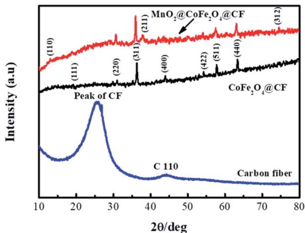
Fig. 4 XRD patterns of CF, CF@CoFe<sub>2</sub>O<sub>4</sub> and CF@CoFe<sub>2</sub>O<sub>4</sub>@MnO<sub>2</sub> composites.
