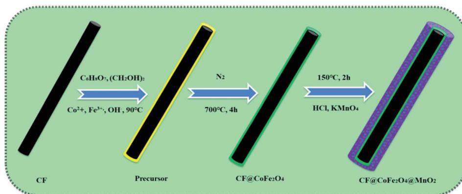
Fig. 1 Explanation of the preparation process of the CF@CoFe<sub>2</sub>O<sub>4</sub>@MnO<sub>2</sub> composite.
