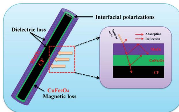
Fig. 10 Mechanism illustration of microwave absorption for the CF@CoFe<sub>2</sub>O<sub>4</sub>@MnO<sub>2</sub> composite.
