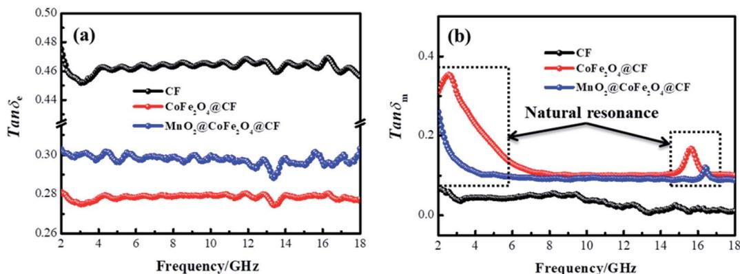
Fig. 8 Dielectric loss (a) and magnetic loss (b) of CF, CF@CoFe<sub>2</sub>O<sub>4</sub> and CF@CoFe<sub>2</sub>O<sub>4</sub>@MnO<sub>2</sub> composites.
