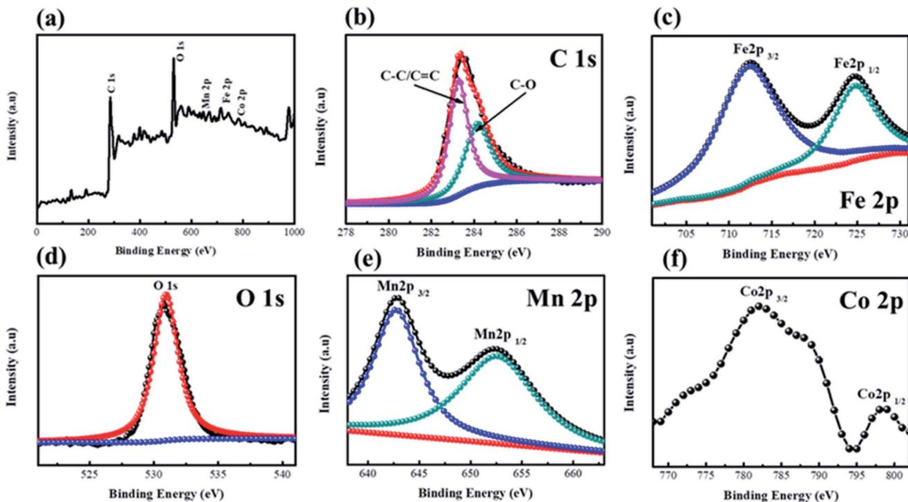
Fig. 5 XPS spectra of CF@CoFe<sub>2</sub>O<sub>4</sub>@MnO<sub>2</sub> composite, a survey scan (a), C 1s (b), Fe 2p (c), O 1s (d), Mn 2p (e), Co 2p (f).
