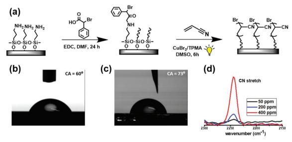
Fig. 2 (a) Schematic illustration of the synthetic route to PAN brushes by photoinduced SI-ATRP; water contact angle before (b) and after (c) coupling BPAA to the APTES-modified silicon wafer; (d) FT-IR spectra of the surface after SI-ATRP with different catalyst loadings.
