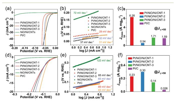
Fig. 5 (a) LSV curves and (b) the corresponding Tafel plots of Pt/NiO/Ni/CNTs, NiO/Ni/CNTs and commercial Pt/C for the HER with iR-compensation in N2-saturated 0.5 M H2SO4 at 1600 rpm. (c)  $J_{mass}$  at  $J_{\eta=50}$  in N2-saturated 0.5 M H2SO4. (d) LSV curves and (e) Tafel plots of Pt/NiO/Ni/CNTs, NiO/Ni/CNTs and commercial Pt/C for the HER with iR-compensation in N<sub>2</sub>-saturated 0.1 M KOH at 1600 rpm. (f)  $J_{mass}$  at  $J_{\eta=50}$  in N<sub>2</sub>-saturated 0.1 м кон.
