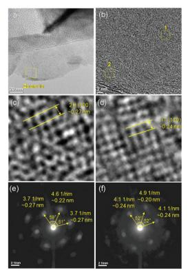
**Fig. 3** (a), (b) High-resolution TEM bright field images of 1T/2H-MoS<sub>2</sub>, (c), (d) zoom in of area 1 and 2 respectively, and (e), (f) selected area electron diffraction (SAED) of area 1 and 2, respectively.
