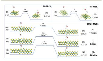
Fig. 8 Geometric structures of the initial state (III) and final state (IV) of the Heryvosky reaction and its energetics on (100)-S atoms of 1T-MoS<sub>2</sub> and 1T/2H interface
