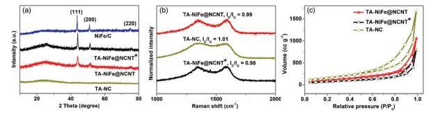
Fig. 2 (a) XRD patterns for TA-NiFe@NCNT, TA-NiFe@NCNT\*, TA-NC, and NiFe/C. (b) Raman spectra, and (c) N2 adsorption and desorption isotherms of TA-NiFe@NCNT, TA-NiFe@NCNT\*, and TA-NC.
