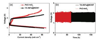
Fig. 6 (a) Charge and discharge polarization curves of rechargeable zinc-air batteries. (b) Charge and discharge cycling curves of rechargeable zinc-air batteries at a current density of 25 mA cm<sup>-2</sup>.
