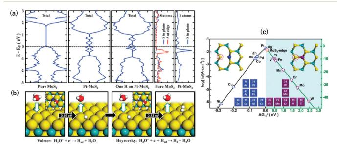
Fig. 2 (a) DOS of MoS<sub>2</sub>, Pt-MoS<sub>2</sub>, and H adsorbed Pt-MoS<sub>2</sub>. The dashed line represents the Fermi level. (b) HER process through the Volmer-Heyrovsky pathway on a Pt-MoS<sub>2</sub> catalyst. (c) Volcano plot of  $2H-MoS_2$  doped with different transition metals at the Mo substitution site.  $^{26}$
