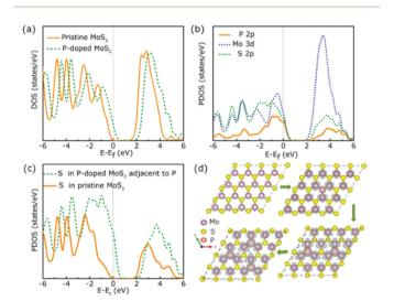
Fig. 5 (a) Total DOS of pure  $MoS_2$  and P doped  $MoS_2$ . (b) Partial DOS of P-MoS<sub>2</sub>. (c) Partial DOS for S atoms. The vertical grey lines represent the Fermi level. (d) Partial charge density of P-MoS<sub>2</sub> when doped with 0–3 P atoms
