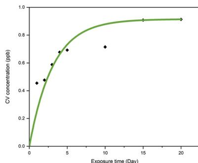
**Fig. 7** The leaching of crystal violet (ppb) from a crystal violet gold nanocluster embedded ultra-high molecular weight polyethylene into phosphate buffer saline solution at room temperature was measured as function of time (day).
