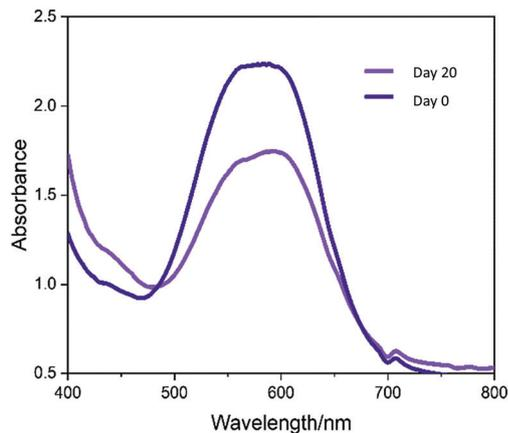
**Fig. 6** UV-Vis spectra measured (400–750 nm) of crystal violet and gold nanocluster compressed moulded UHMWPE. The sample was stored in a light box with constant white light striking on the sample surfaces. The UV-vis absorbance was measured on day 1 and day 20 to investigate the photostability of the material after light exposure for an extended period.
