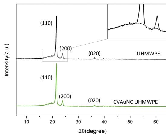
Fig. 2 X-Ray diffraction plots of ultra-high molecular weight polyethylene control and crystal violet embedded ultra-high molecular weight polyethylene sample measured across  $2\theta$  range from 6 to 66°. A small section of the diffraction pattern of the UHMWPE was shown by a zoomed inset shown on the top right.
