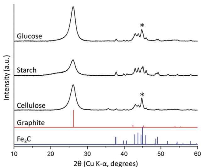
Fig. 2 PXRD patterns for carbon/Fe<sub>3</sub>C samples produced from glucose, starch and cellulose (5 g) and iron nitrate (0.68 mmol), held at 800 °C for 1 h. (\*) indicates presence of minor  $\alpha$ -Fe phase.
