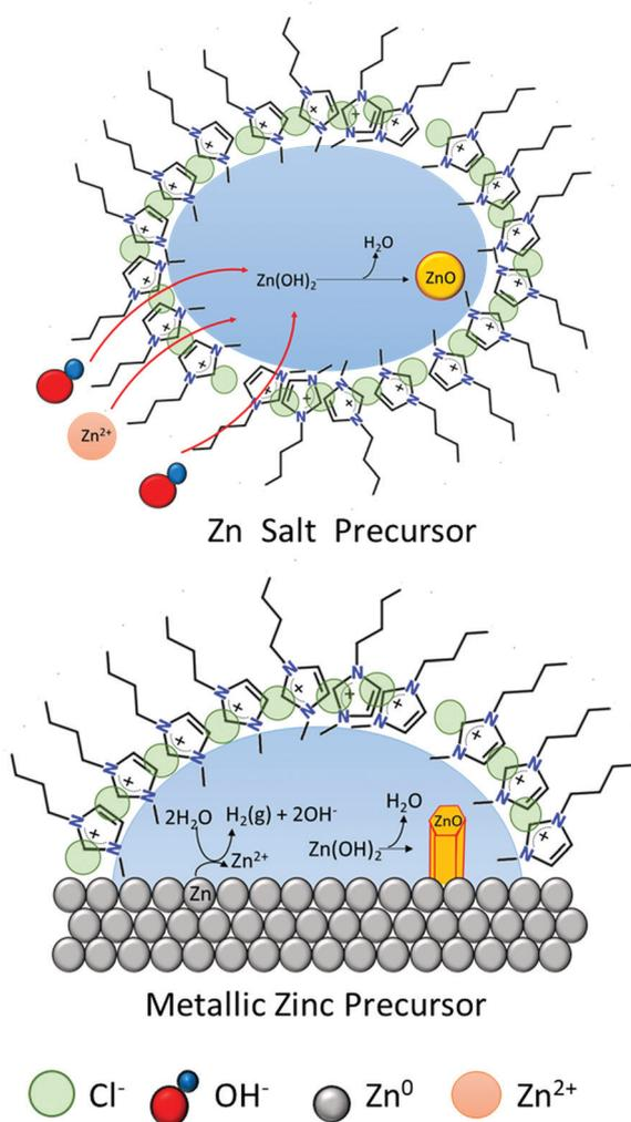
Fig. 8 Schematic of ZnO formation in [C<sub>4</sub>C<sub>1</sub>im]Cl at low water content. Left: Zn salts as precursors.<sup>40</sup> Right: Metallic zinc as precursor.
