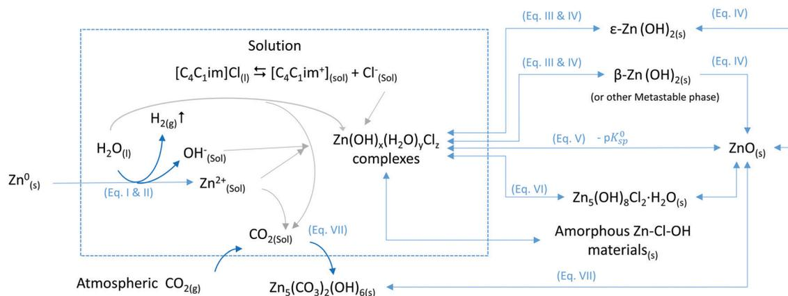
Fig. 9 General conversion paths of metallic zinc into ZnO in [C<sub>4</sub>C<sub>1</sub>im]Cl/water systems. Equations in the scheme are not balanced. Equations are given in the text. The predominant path and species formed will depend on the temperature and water content.
