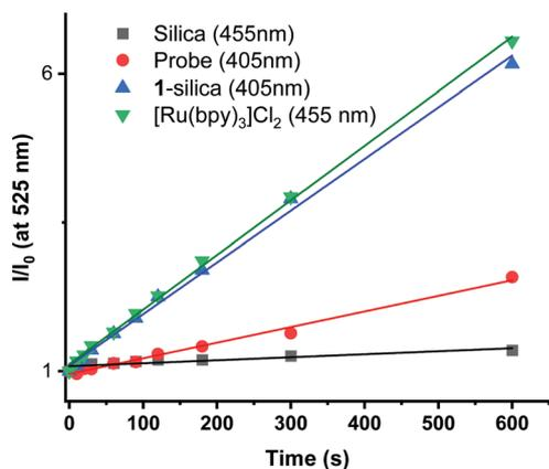
Fig. 3 Relative emission intensity of SOSG probe ( $\lambda_{\text{max}} = 525 \text{ nm}$ ) in water as a function of irradiation time. Probe (1 nM, -square-),  $[\text{Ru}(\text{bpy})_3]\text{Cl}_2$  in solution (1.56  $\mu\text{M}$ , -upside down triangle-); silica suspension (5 mg  $\text{ml}^{-1}$ , -circle-); **1**-silica suspension (5 mg  $\text{ml}^{-1}$ , 55  $\mu\text{M}$ , -triangle-).
