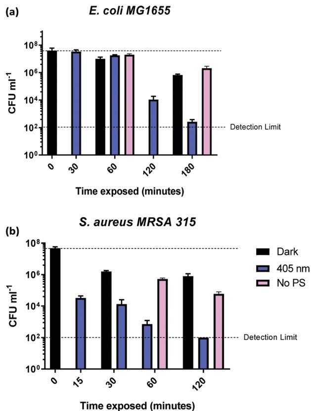
Fig. 6 Colony forming units (CFU ml<sup>-1</sup>) for (a) *E. coli* MG1655 and (b) *S. aureus* MRSA 315, in presence of 5 mg ml<sup>-1</sup> of **1**-silica as a function of irradiation time with 405 nm light, 17.5 mW cm<sup>-2</sup> (blue bars) and in the absence of 5 mg ml<sup>-1</sup> of **1**-silica (pink bars).
