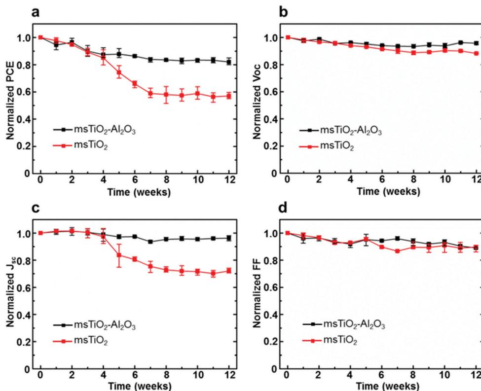
Fig. 2 Evolution of photovoltaic parameters: (a) PCE, (b)  $V_{\text{oc}}$ , (c)  $J_{\text{sc}}$ , and (d) FF of the PSCs based on different mesoporous scaffolds stored in ambient air at >65% relative humidity. The measurement was carried out immediately after fabrication and once a week in the following 12 weeks. Each value is the average over 8 cells in the same counterparts.
