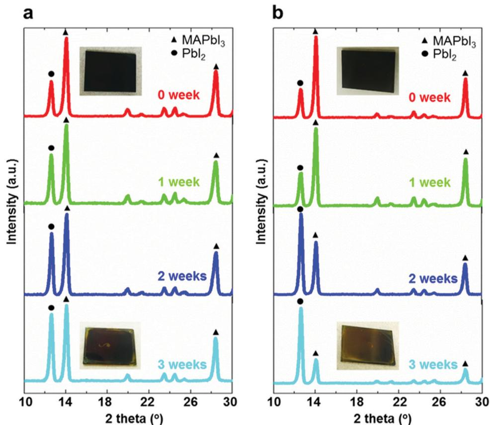
Fig. 3 XRD spectra in the  $2\theta$  range from 10° to 30° of the perovskite films based on (a) the bilayer mesoporous scaffold and (b) the single mesoporous scaffold after different aging times in ambient air at >65% relative humidity. The insets are the top views of the corresponding perovskite films.
