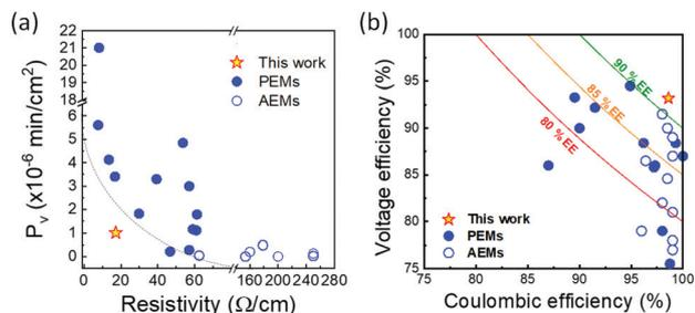
Fig. 4 (a) Trade-off between vanadium diffusivity and resistivity. (b) VRFB performance relationship among CE, VE, and EE at  $40\text{--}60 \text{ mA cm}^{-2}$ . Detailed information on the trade-off curves is available in Tables S3 and S4 (ESI<sup>†</sup>).
