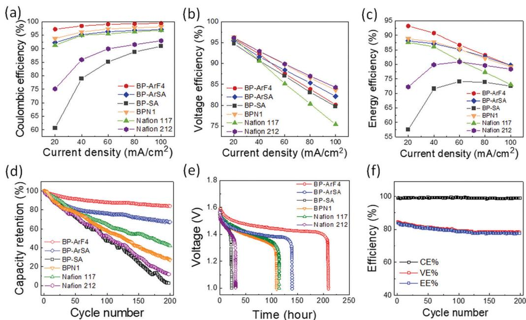
Fig. 2 VRFB single cell performance. (a) CE for PEMs at a current density from  $20$  to  $100 \text{ mA cm}^{-2}$ , (b) VE for PEMs at a current density from  $20$  to  $100 \text{ mA cm}^{-2}$ , (c) EE for PEMs at a current density from  $20$  to  $100 \text{ mA cm}^{-2}$ , (d) capacity retention for IEMs at  $100 \text{ mA cm}^{-2}$ , (e) self-discharge curves of PEMs, and (f) cycling stability of VRFB with the **BP-ArF4** membrane at  $100 \text{ mA cm}^{-2}$ .
