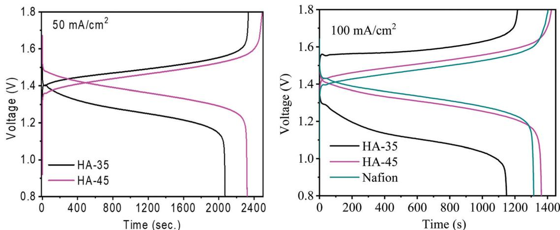
**Fig. 4** Charging and discharging for single cell VRFB with HA-35, HA-45 and Nafion 117 membrane at 50 mA cm<sup>-2</sup> and 100 mA cm<sup>-2</sup> current density.
