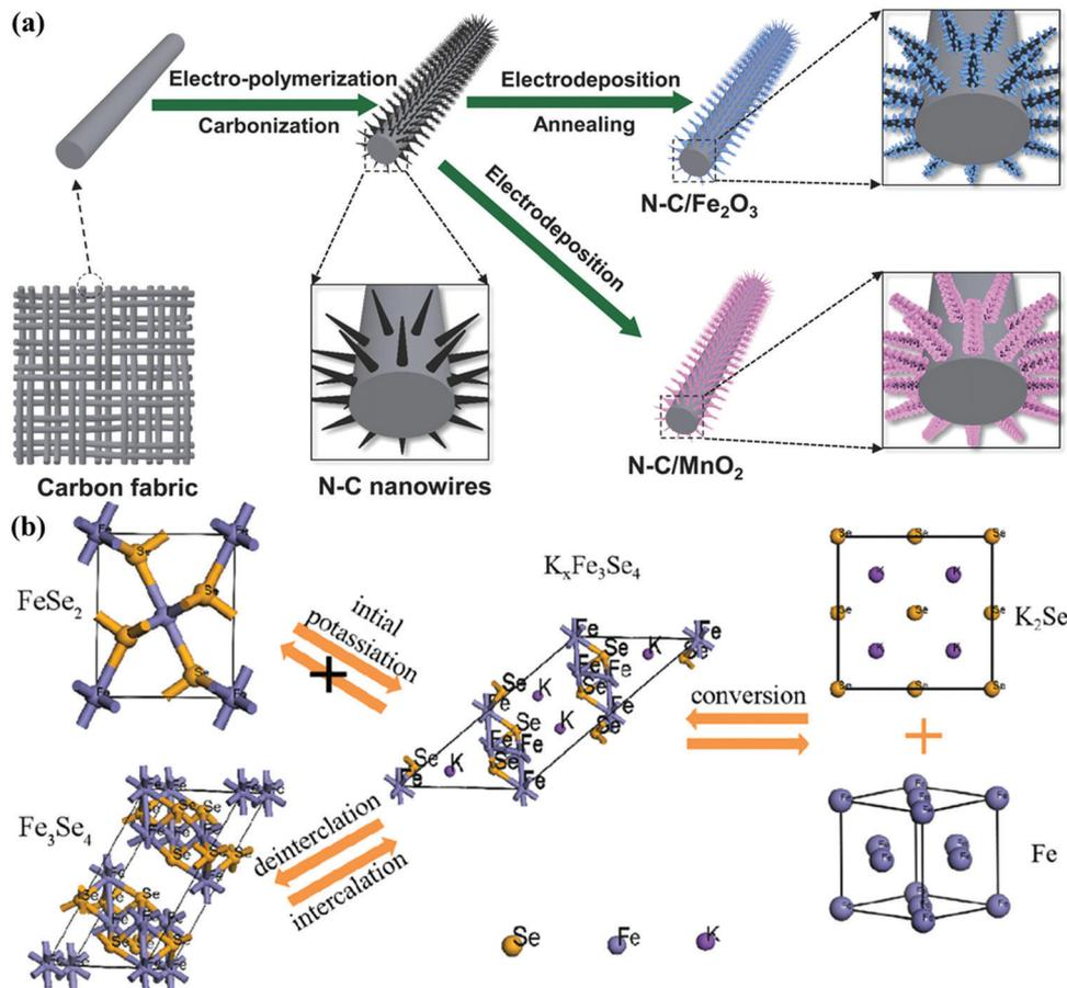
Fig. 10 Schematic of N-doped carbon nanowires@MnO<sub>2</sub> and N-doped carbon nanowires@Fe<sub>2</sub>O<sub>3</sub> (a). (Reproduced with permission.<sup>147</sup> Copyright 2018, Wiley-VCH.) Schematic for the potassium storage reaction mechanism (b). (Reproduced with permission.<sup>157</sup> Copyright 2019, Wiley-VCH.)
