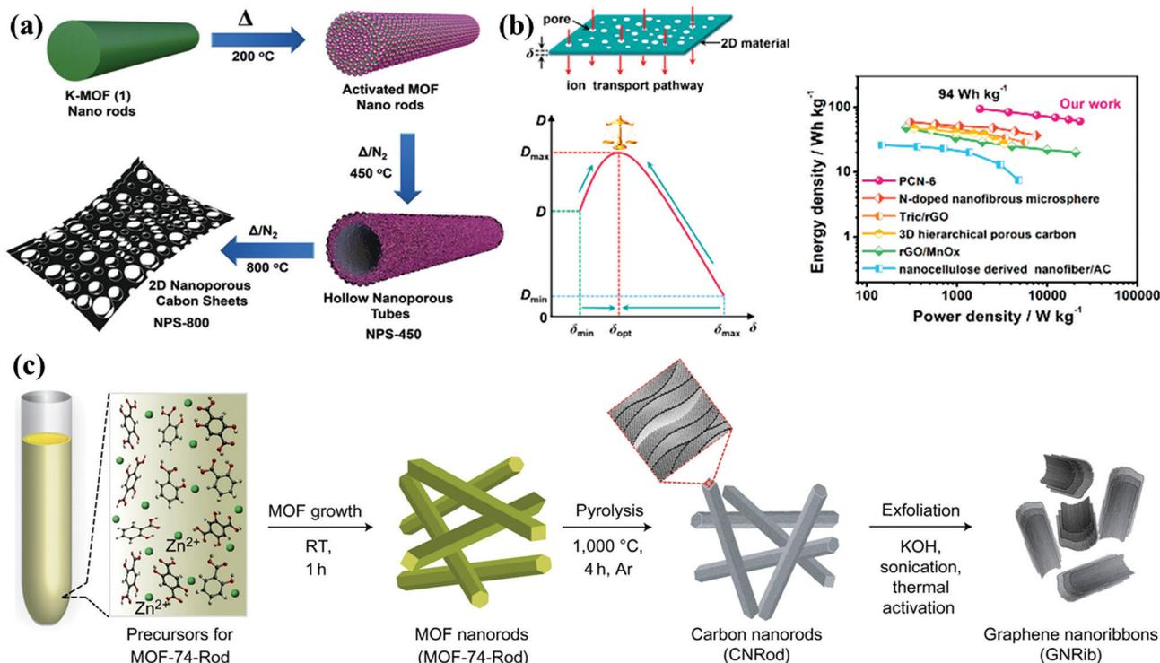
Fig. 4 Synthesis of MOF-based 2D carbon nanosheets (a). (Reproduced with permission.<sup>43</sup> Copyright 2018, Wiley-VCH.) Schematic illustration of ion transfer inside a 2D carbon electrode; correlation between the sheet thickness and ion transport behavior; and Ragone plots (b). (Reproduced with permission.<sup>46</sup> Copyright 2019, Elsevier.)
