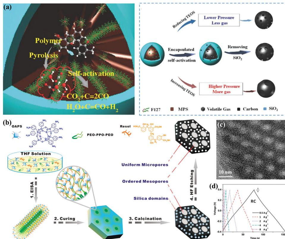
Fig. 7 Schematic illustration of monodispersed mesoporous carbon spheres (a). (Reproduced with permission.<sup>85</sup> Copyright 2018, Wiley-VCH.) Schematic illustration of ordered mesoporous carbons (b). TEM image (c). Galvanostatic charge/discharge curves (d). (Reproduced with permission.<sup>98</sup> Copyright 2016, Elsevier.)
