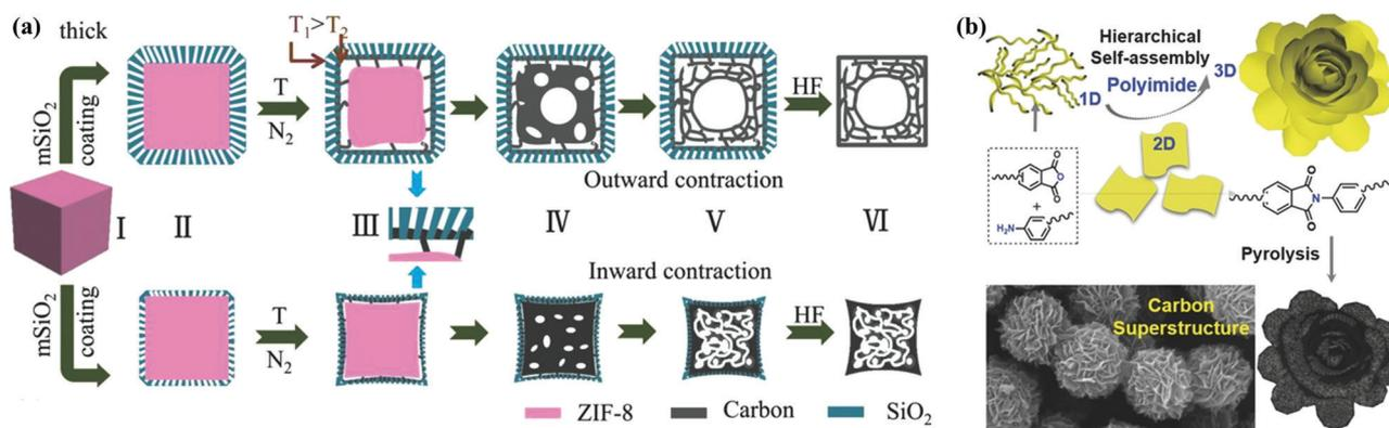
Fig. 5 Schematic illustration of hollow mesoporous carbon nanocubes (a). (Reproduced with permission.<sup>58</sup> Copyright 2017, Wiley-VCH.) Fabrication scheme of porous carbon superstructures (b). (Reproduced with permission.<sup>65</sup> Copyright 2016, Wiley-VCH.)
