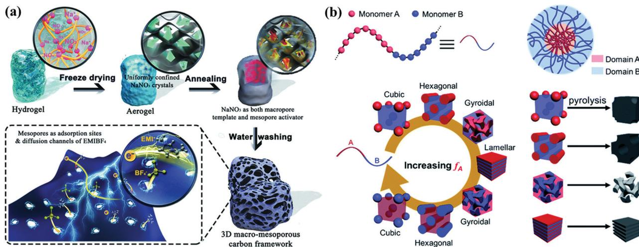
Fig. 8 Schematic illustration of the synthesis of hierarchical porous carbons from a gelatin– $\text{NaNO}_3$  biopolymer (a). (Reproduced with permission.<sup>104</sup> Copyright 2018, Wiley-VCH.) Examples of porous carbon structures after the calcination of block copolymers (b). (Reproduced with permission.<sup>92</sup> Copyright 2019, The Royal Society of Chemistry.)
