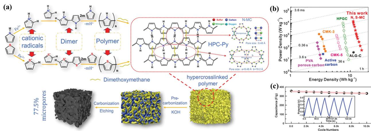
Fig. 6 Synthesis of hypercrosslinked polymer-derived carbons (a). Ragone plots (b). Long-term cycling performance (c). (Reproduced with permission.<sup>78</sup> Copyright 2019, Elsevier.)
