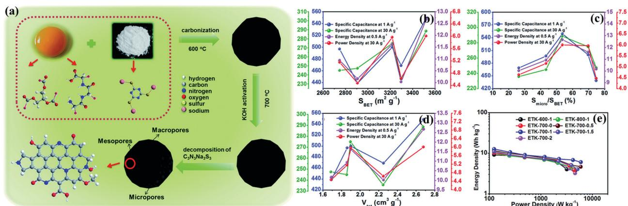
Fig. 2 Schematic of the preparation of egg yolk-derived activated carbons (a). Influence among the structural parameters, *i.e.*,  $S_{\text{BET}}$  (b);  $S_{\text{micro}}/S_{\text{BET}}$  (c);  $V_{\text{tot}}$  (d); and electrochemical performances such as specific capacitance, power density, energy density, and rate density. Ragone plots (e). (Reproduced with permission.<sup>30</sup> Copyright 2018, The Royal Society of Chemistry.)
