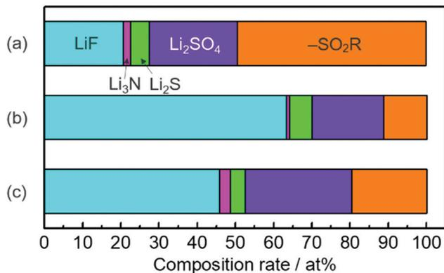
Fig. 6 Chemical species and their composition rates, estimated from XPS data, contained in SEI films formed during the charge process in (a) 83.3–16.7 mol% [C<sub>2</sub>mim][FSA]–Li[TFSA], (b) 83.3–16.7 mol% [C<sub>2</sub>mim][FSA]–Li[FSA] and (c) 50.0–50.0 mol% [C<sub>2</sub>mim][FSA]–Li[FSA] IL electrolytes.
