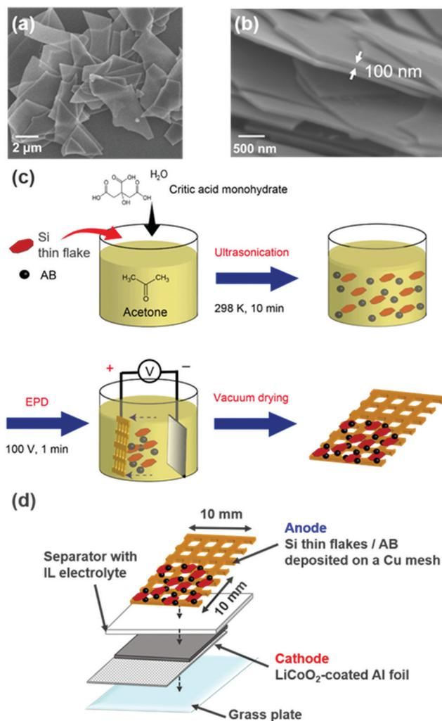
Fig. 1 SEM images of (a) top view and (b) cross-sectional view of the Si thin flakes. Schematic drawings of (c) a binder-free Si anode preparation process and (d) an *operando* SEM observation cell for the binder-free Si anode reaction.
