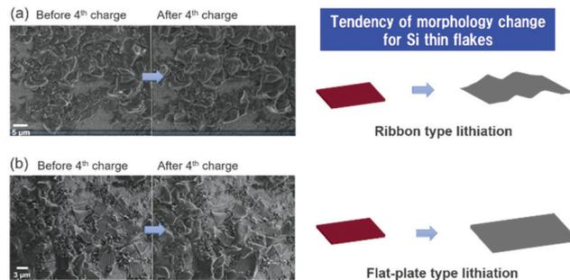
Fig. 7 SEM images of the binder free Si thin flake anode in the *operando* SEM observation cell before and after the fourth charge process. The test was conducted at a CC/CV mode. The CC rate was 1/2C and the cut-off voltages were –3.88 V and –2.40 V (vs. LiCoO<sub>2</sub>). The cut-off current density was 1/20C. The electrolytes were (a) 83.3–16.7 mol% [C<sub>2</sub>mim][FSA]–Li[TFSA] and (b) 83.3–16.7 mol% [C<sub>2</sub>mim][FSA]–Li[FSA].
