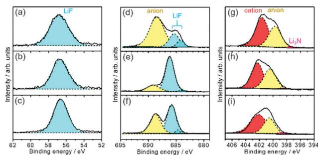
**Fig. 5** XPS spectra for (a–c) Li-1s, (d–f) F-1s, and (g–i) N-1s of the Si thin flake composite anodes after five charge–discharge cycles. The charge–discharge test was conducted in a CC mode at 1/2C, and the cut-off voltages were  $-3.88$  V and  $-2.40$  V (vs. LiCoO<sub>2</sub>). The IL electrolytes were (a, d and g) 83.3–16.7 mol% [C<sub>2</sub>mim][FSA]–Li[TFSA], (b, e and h) 83.3–16.7 mol% [C<sub>2</sub>mim][FSA]–Li[FSA], and (c, f and i) 50.0–50.0 mol% [C<sub>2</sub>mim][FSA]–Li[FSA].
