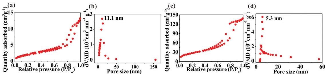
Fig. 4 Nitrogen adsorption-desorption isotherms and pore-size distribution of TiO<sub>2</sub>/C (a and b) and SnO<sub>2</sub>@TiO<sub>2</sub>/C (c and d).
