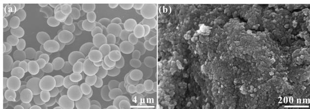
Fig. 1 SEM images of TiO<sub>2</sub>/C (a) and SnO<sub>2</sub>@TiO<sub>2</sub>/C (b).
