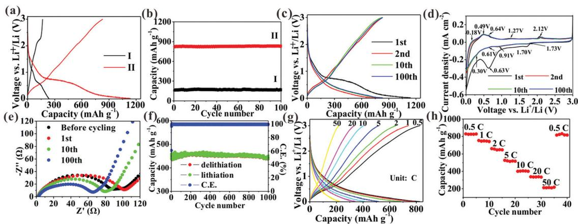
Fig. 5 (a) First charge/discharge curves; (b) cycling curves at 0.5C of TiO<sub>2</sub>/C (I) and SnO<sub>2</sub>@TiO<sub>2</sub>/C (II); (c) charge/discharge curves at different cycles; (d) CV curves; (e) Nyquist plots; (f) cycling performance at 10C; (g) charge/discharge curves at different current densities; and (h) rate performance of SnO<sub>2</sub>@TiO<sub>2</sub>/C.
