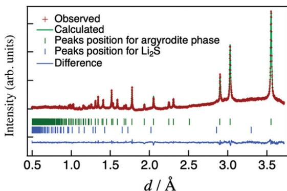
Fig. 4 Neutron-diffraction Rietveld-refined patterns for  $\text{Li}_{6.15}\text{Al}_{0.15}\text{Si}_{1.35}\text{S}_{5.4}\text{O}_{0.6}$ .
