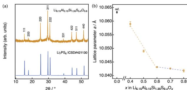
Fig. 2 (a) X-ray diffraction pattern for  $\text{Li}_{6.15}\text{Al}_{0.15}\text{Si}_{1.35}\text{S}_{5.4}\text{O}_{0.6}$  along with the pattern of argyrodite  $\text{Li}_7\text{PS}_6$  (ICSD: 421130), which is indexed as the cubic argyrodite phase. (b) Lattice parameter for  $\text{Li}_{6.15}\text{Al}_{0.15}\text{Si}_{1.35}\text{S}_{6-x}\text{O}_x$  as a function of the nominal oxygen content  $x$ . The lattice data for  $x = 0$  are taken from the literature.<sup>25</sup>
