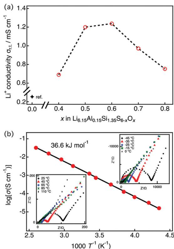
Fig. 3 (a) Lithium ion conductivity of LASSO as a function of the nominal  $x$ , as obtained by impedance spectroscopy at  $25$  °C. The conductivity data for  $x = 0$  was obtained from the literature.<sup>25</sup> (b) Impedance plots for conductivity data between  $-45$  and  $110$  °C (insets) and the Arrhenius plot for  $\text{Li}_{6.15}\text{Al}_{0.15}\text{Si}_{1.35}\text{S}_{5.4}\text{O}_{0.6}$ . Conductivities were obtained by summing the grain-boundary and bulk resistances.
