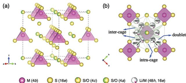
Fig. 5 (a) The  $\text{Li}_{6.15}\text{Al}_{0.15}\text{Si}_{1.35}\text{S}_{5.4}\text{O}_{0.6}$  framework with the HT-argyrodite-type structure ( $\text{M} = \text{Al}_{0.1}\text{Si}_{0.9}$ ). (b) Lithium diffusion pathways, showing three types of Li migration: doublet (solid line), intra-cage (dashed line), and inter-cage (dotted line).
