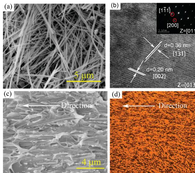
Fig. 2 (a) SEM image of BaTiO<sub>3</sub> nanowires; (b) HRTEM image of a single BaTiO<sub>3</sub> nanowire; (c) SEM and (d) POM images of nanocomposites prepared by 3D printing with 5 vol% aligned BaTiO<sub>3</sub> nanowires.
