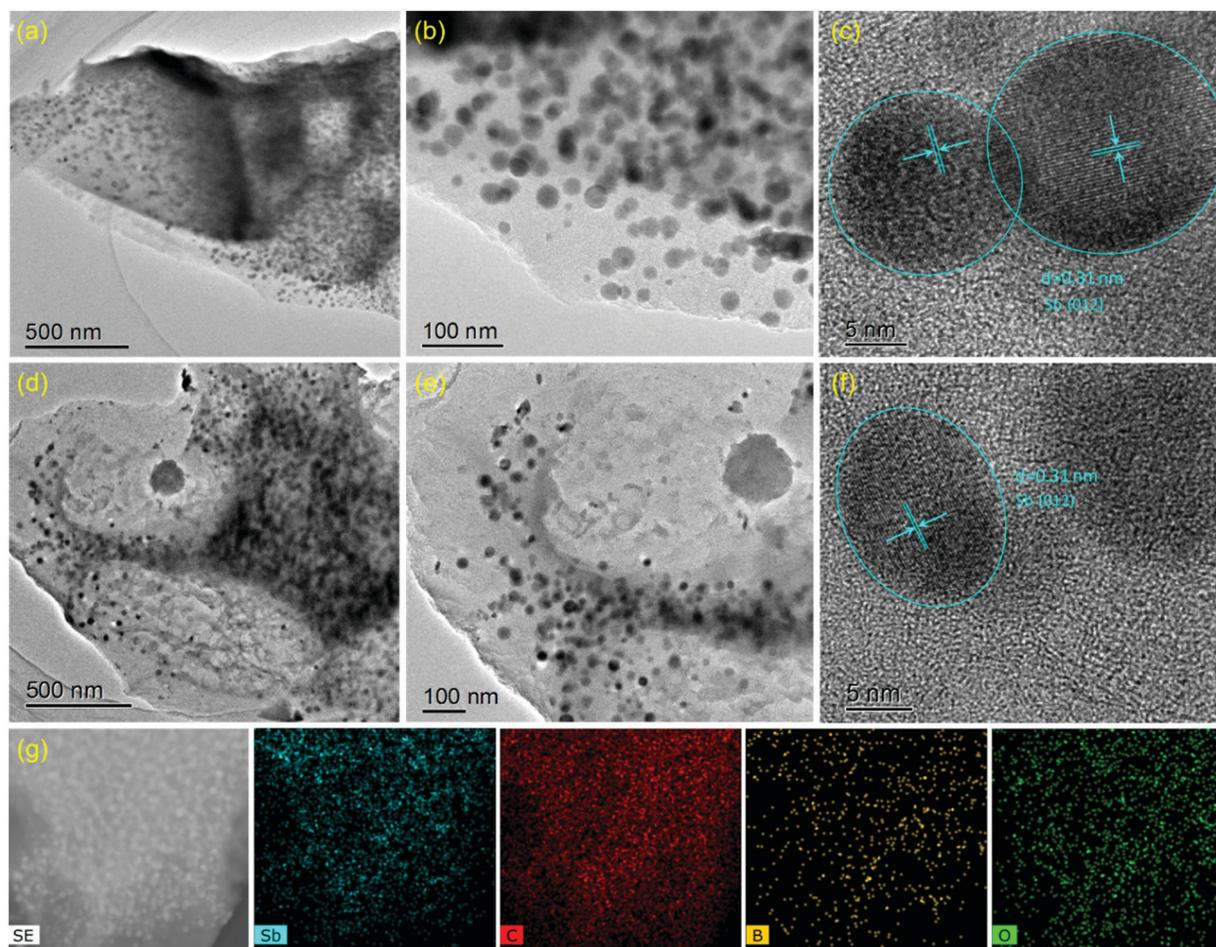
Fig. 2 TEM images (a and b) and HRTEM images (c) of the  $\text{Sb}/\text{BC}_x$  composite; TEM images (d and e) and HRTEM images (f) of the  $\text{Sb}/\text{C}$  composite; (g) scanning TEM image with its corresponding EDS mappings of the Sb, C, B and O elements for the  $\text{Sb}/\text{BC}_x$  composite.
