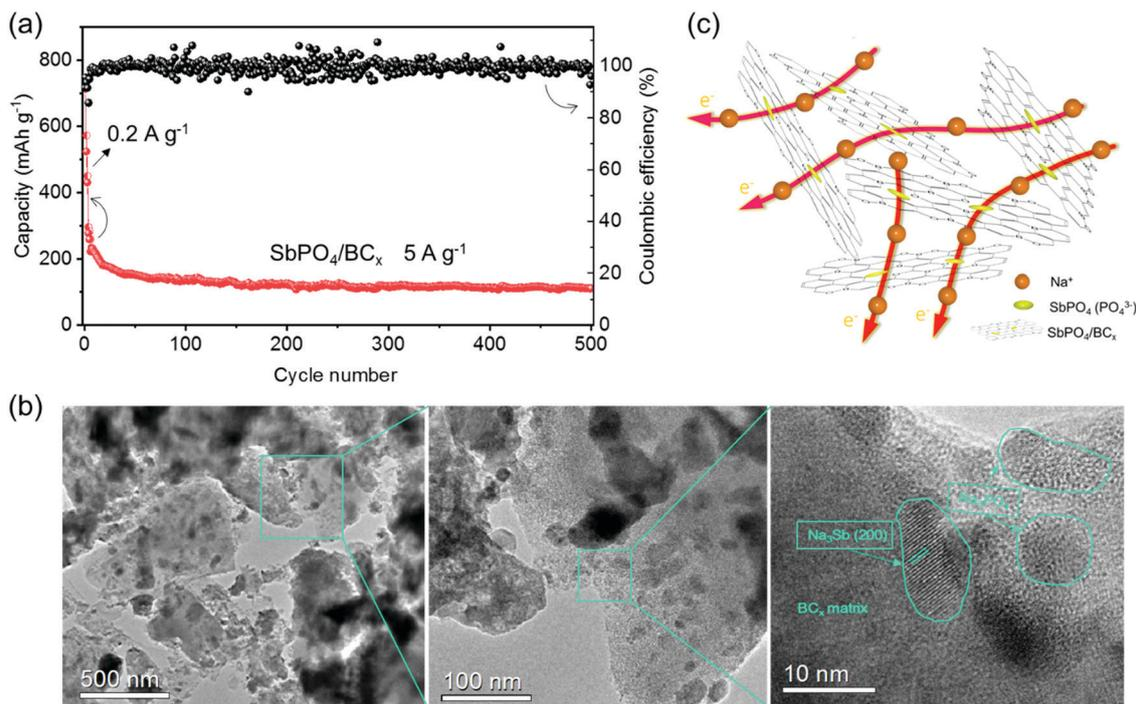
Fig. 6 (a) Cycling performance of the  $\text{SbPO}_4/\text{BC}_x$  electrode at  $5 \text{ A g}^{-1}$  after three cycles at  $0.2 \text{ A g}^{-1}$ . (b) TEM images of the  $\text{SbPO}_4/\text{BC}_x$  electrode after 500 cycles. (c) Proposed mechanism of the  $\text{SbPO}_4/\text{BC}_x$  composite during the sodium storage processes.
