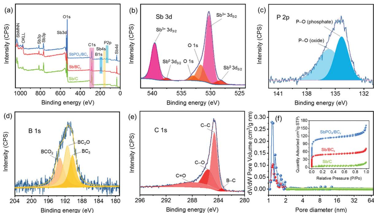
Fig. 4 (a) XPS survey of  $SbPO_4/BC_x$ ,  $Sb/BC_x$  and  $Sb/C$ , and the fitted Sb 3d signal (b), P 2p signal (c), B 1s signal (d), and C 1s signal (e) for the  $SbPO_4/BC_x$  composite. (f) NLDFT adsorption pore size distribution plots (the inset presents  $N_2$  adsorption–desorption isotherm curves) of the  $SbPO_4/BC_x$ ,  $Sb/BC_x$  and  $Sb/C$  samples.
