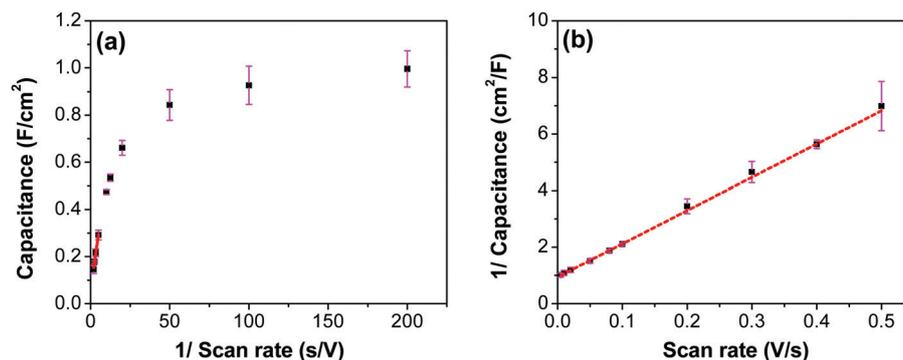
Fig. 14 (a) Capacitance as a function of the inverse of scan rate for the RuO<sub>2</sub>-CNF electrodes prepared at 250 °C. (b) The inverse of capacitance as a function of scan rate. Red line indicates linear fit with the equation (a)  $y = 0.05x + 0.06$ , and (b)  $y = 11.76x + 0.94$ .
