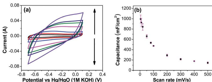
Fig. 13 (a) CV curves of RuO<sub>2</sub>-CNF prepared at 250 °C recorded in a three-electrode cell at scan rates of 5, 10, 20, 50, 80, 100, 200 mV s<sup>-1</sup> (the scan rate increases in the direction of the arrows). (b) Change in capacitances with scan-rate (capacitance values are reported per electrode).
