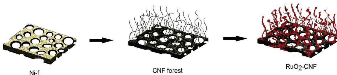
Fig. 1 Schematic of the electrode preparation, from Ni-f to RuO<sub>2</sub>-CNF.
