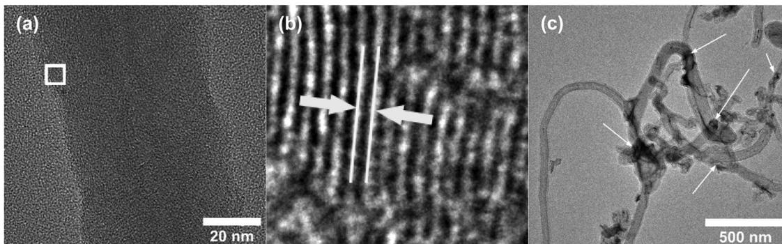
**Fig. 3** (a) HR-TEM image of uncoated CNF showing a large number of zones having graphitic layer structures when viewed in high resolution, (b) enlarged image of the white-box in Fig. 3a, showing one example of such zone. The white lines and the arrow depict the spacing between the graphitic layers, which is found to be ca. 0.34 nm, characteristic of graphite. (c) TEM image of RuO<sub>2</sub>-CNF electrode prepared at 250 °C. Arrows show some RuO<sub>2</sub> sheets (dark regions).
