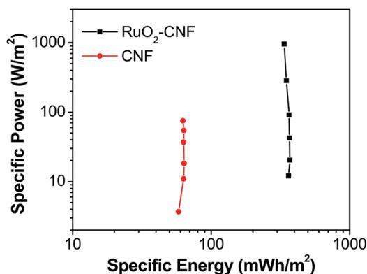
Fig. 11 Ragone plot comparing the performance of RuO<sub>2</sub>-CNF electrode prepared at 250 °C (present work) to the uncoated-CNF electrode.<sup>6</sup>
