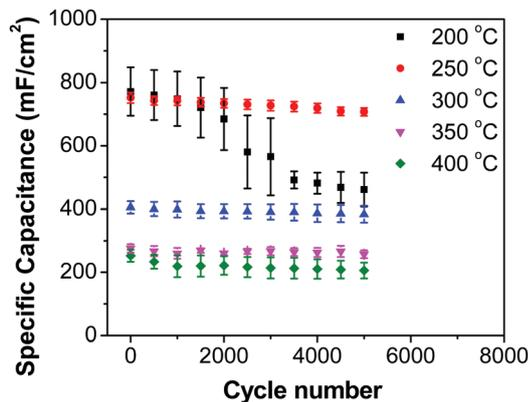
Fig. 15 Specific capacitances at different GCD cycle numbers for various RuO<sub>2</sub>-CNF electrodes measured at 200 mA/cm<sup>2</sup>.
