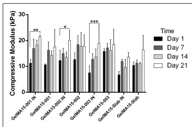
Fig. 6 Compressive moduli change of cell loaded IN 3D printed, unloaded 3D printed, cell loaded GelMA15-Slab and unloaded GelMA15-Slab hydrogels over 3 weeks. IN: with cells. \* $p < 0.05$ , \*\* $p < 0.01$ , and \*\*\* $p < 0.001$ .
