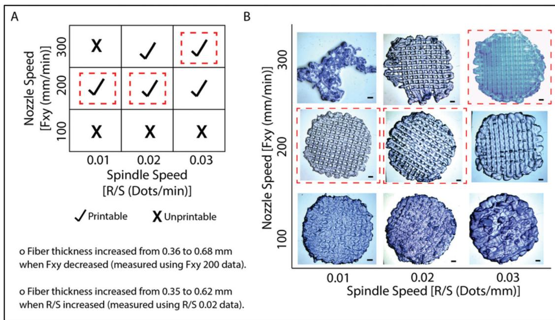
**Fig. 2** Printing conditions and appearance of 3D printed GelMA hydrogels. (A) Print condition optimization of the hydrogels under varying conditions of speed of the nozzle in the  $x$ - $y$  direction (Fxy,  $\text{mm min}^{-1}$ ) and spindle speed (R/S, dots per min). Dotted red lines indicate parameters selected for use in the following studies. (B) Stereomicrographs of the hydrogels. The scale bar is 1 mm.
