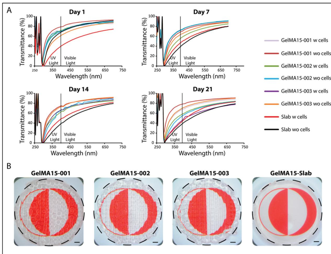
**Fig. 9** Light transmission of the 3D printed hydrogels. (A) Change of transparency of the cell free and keratocyte carrying hydrogels with incubation time. (B) Stereomicrographs showing transparency of cell free hydrogels on day 0 (outlined in black). The scale bar is 1 mm. w: with, wo: without.
