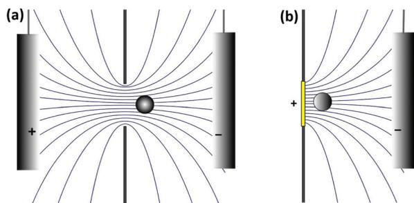
**Fig. 5** Schematic representation of the analogy between the Coulter counter and current blockade. (a) Electric field lines are distorted by the presence of a particle in the Coulter counter, leading to a change in migrational current. (b) The diffusive flux of the redox mediator is distorted in a similar manner during current blockade.
