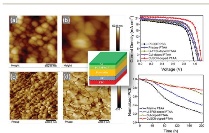
Fig. 10 AFM height and phase images of the perovskite films on different PTAA layers: (a and c) pristine, (b and d) CuSCN-doped cases; (right)  $J$ - $V$  curves of the PSCs based on pristine and doped PTAA as HTLs (up) and normalized PCE (down) of the PSCs based on pristine and doped PTAA for 200 h. (central image) Device architecture<sup>98</sup> (reprinted (adapted) with permission from *ACS Appl. Energy Mater.*, 2019, **23**, 1932–1942, Copyright 2019 American Chemical Society).
