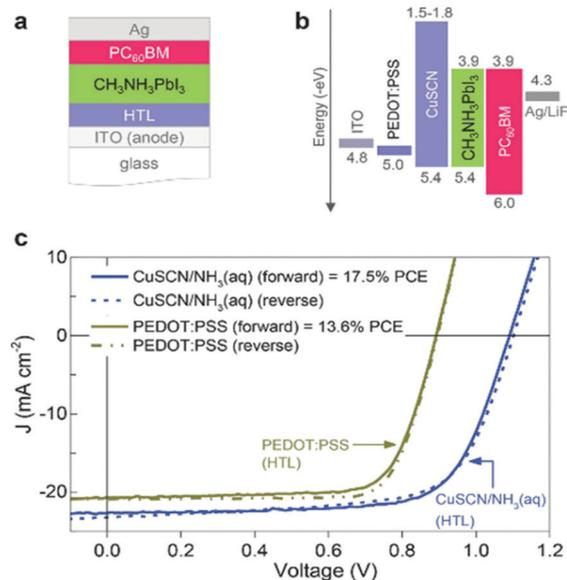
Fig. 6 (a) Schematic cross-section of the cell architecture employed; (b) corresponding material energetics; and (c)  $J$ - $V$  characteristics measured under simulated 1 sun solar illumination for the champion  $\text{CH}_3\text{NH}_3\text{PbI}_3$  solar cells based on CuSCN/ $\text{NH}_3$  (aq) and PEDOT:PSS HTLs.<sup>90</sup>
