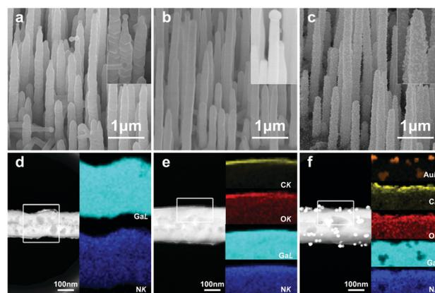
**Fig. 2** Representative  $40^\circ$ -tilted SEM images for (a) GaN nanowire array, (b) GaN nanowire array/PDA and (c) GaN nanowire array/PDA/Au NPs; insets display the morphology of individual nanowires after each assembly step. STEM images for an individual nanowire after each step and its corresponding spatially resolved elemental mapping are shown in (d–f), respectively. The selected areas for compositional analysis are marked by white squares at the left side.
