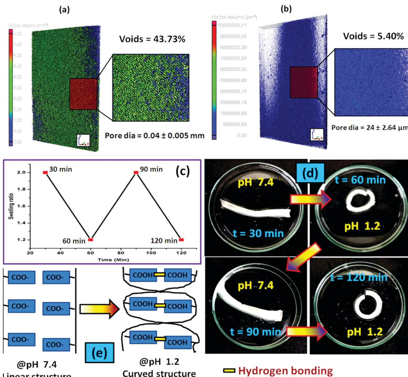
Fig. 8 Micro CT analysis of the hydrogel having a composition of (a) PSAS<sub>50</sub>C<sub>0</sub> and (b) PSAS<sub>50</sub>C<sub>5</sub>; (c) actuation cycle of the composite hydrogel (PSAS<sub>50</sub>C<sub>5</sub>) in the presence of acid (pH 1.2); (d) acid induced actuation in the composite hydrogel system (PSAS<sub>50</sub>C<sub>5</sub>) and (e) probable mechanism lying behind the actuation.
