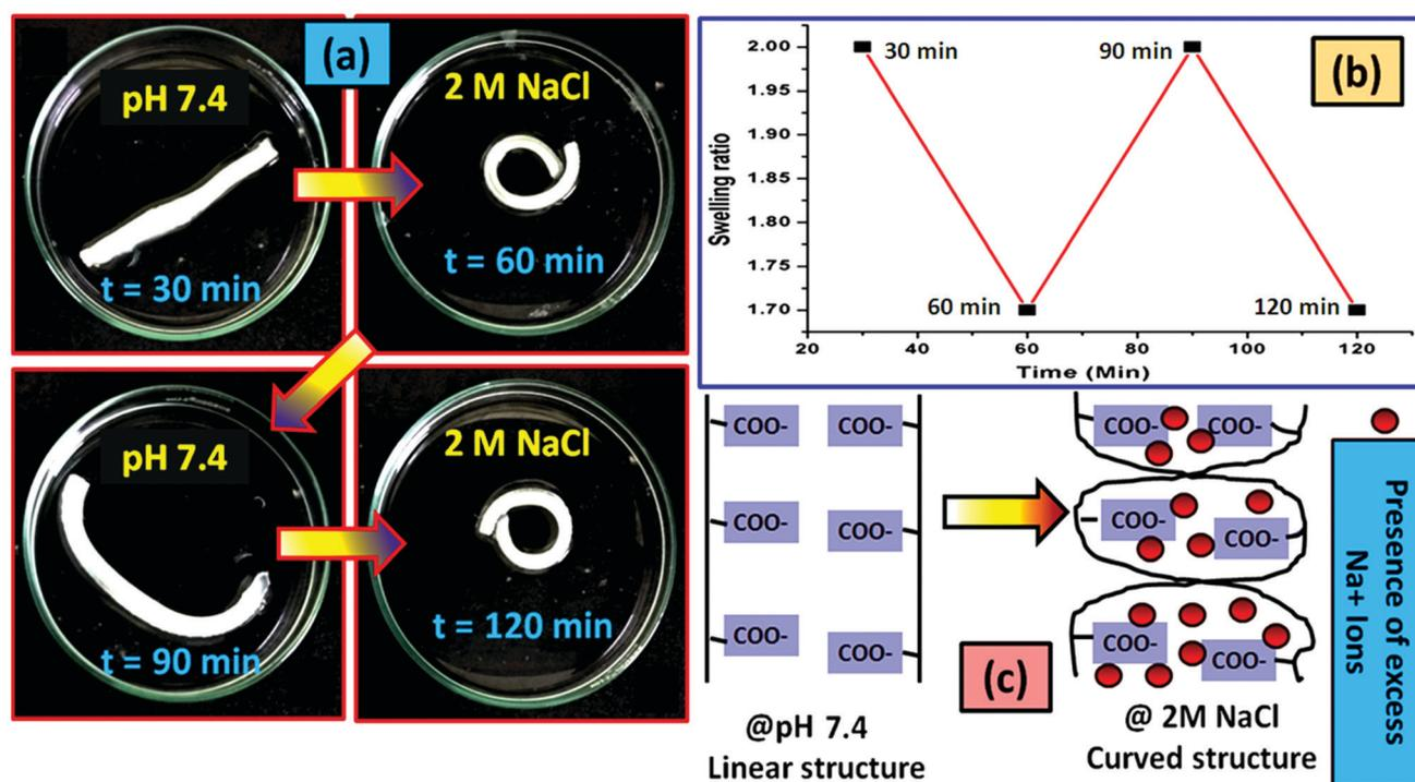
Fig. 9 (a) Salt induced actuation in the composite hydrogel system (PSAS<sub>50</sub>C<sub>5</sub>), (b) actuation cycle of the composite hydrogel (PSAS<sub>50</sub>C<sub>5</sub>) in the presence of NaCl solution (2 M, a typical concentration) and (c) probable mechanism lying behind the actuation.
