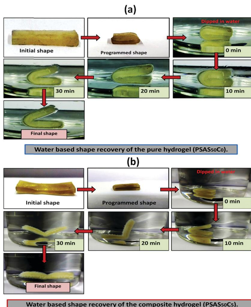
Fig. 7 Water-based shape recovery study over the (a) single component hydrogel (PSAS<sub>50</sub>C<sub>0</sub>) and (b) composite hydrogel (PSAS<sub>50</sub>C<sub>5</sub>).
