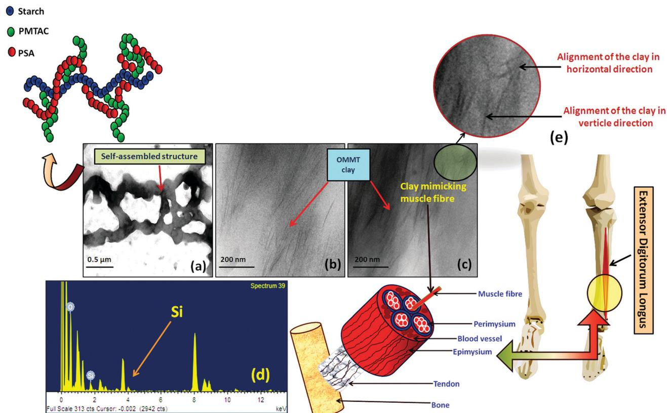
Fig. 2 HRTEM images of (a) the self-assembled structure of cationic starch and anionic pol(sodium acrylate); (b and c) composite hydrogel with 5.0 wt% (PSAS<sub>50</sub>C<sub>5</sub>) and 7.0 wt% (PSAS<sub>50</sub>C<sub>7</sub>) of OMMT; (d) EDAX analysis of the composite hydrogel containing 5 wt% of filler (PSAS<sub>50</sub>C<sub>5</sub>) and (e) schematic of the location of EDL muscle present in the human body.
