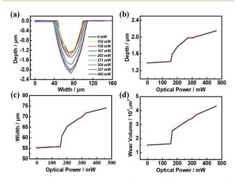
Fig. 5 (a) Cross-sectional profiles, (b) depths, (c) widths, and (d) removal volumes of the concave microlens fabricated on an n-GaAs wafer under different illumination powers. The imprint time is 15 minutes, and the aqueous solution contains 40 mM KMnO $_4$  and 1.84 M  $H_2$ SO $_4$ .
