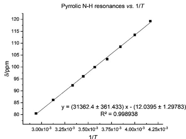
Fig. 7 Temperature dependence of pyrrole <sup>1</sup>H NMR spectroscopic resonance in **8** between 240 K and 340 K.
