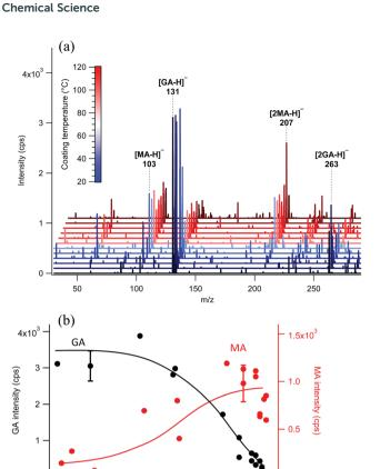
Fig. 5 EASI-MS orthogonal mode analysis of polydisperse glutaric acid (GA) particles coated with malonic acid (MA) at increasing coating reservoir temperatures. (a) EASI-MS spectra collected in orthogonal mode. Spectra were averaged over approximately one minute. (b) Signal intensities of GA (black) and MA (red) as a function of MA coating temperature. Error bars represent 1s standard deviations and the solid lines are guidelines only.
