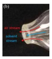
Fig. 1 Easy ambient sonic-spray ionization nebulizer (a) schematic (not to scale) and (b) photograph of the nebulizer tip.
