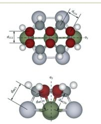
Fig. 5 Naming of the C-C and M-C bonds of nap-di-bridge[7] on Pt(111).  $\eta^2$ -Coordinated C are labelled in red, and the dashed lines label the  $\sigma_2$  mirror plane which bisects every  $\eta^2$ -coordinated C-C bonds. For clarity, we show just the Pt atoms that are binding with C atoms.
