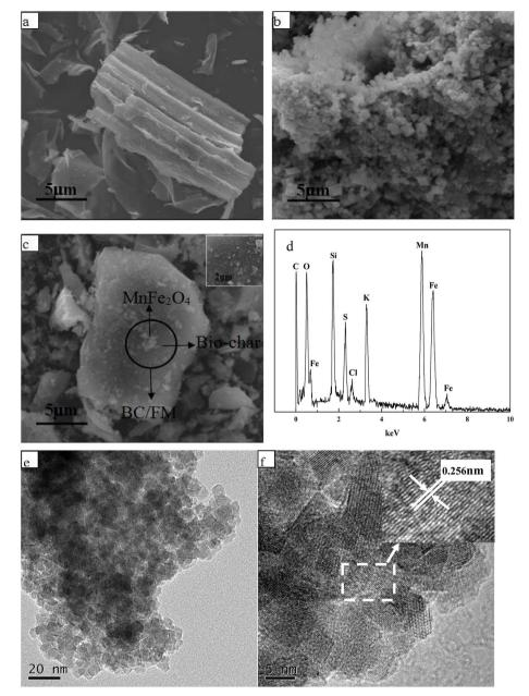
Fig. 2 SEM image of (a) BC, (b) MnFe<sub>2</sub>O<sub>4</sub>, (c) BC/FM; (d) EDS analysis of BC/FM; (e) TEM image and (f) HRTEM image of BC/FM.
