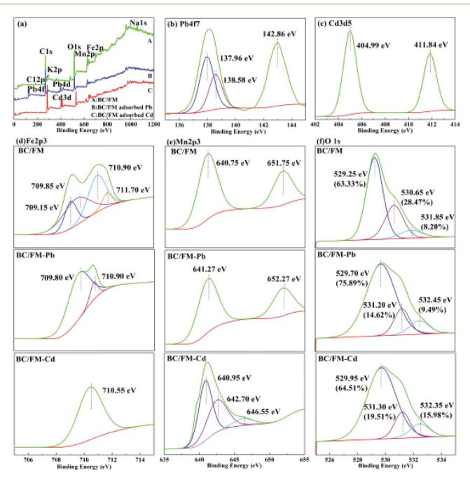
Fig. 10 XPS spectra of BC/FM before and after adsorption for Pb(II) and Cd(III). (a) XPS spectra of BC/FM before and after Pb(II) and Cd(III) adsorption; (b) Pb 4f XPS spectra of BC/FM-Pb; (c) Cd 3d XPS spectra of BC/FM-Cd; (d) Fe 2p XPS spectra of BC/FM, BC/FM-Pb and BC/FM-Cd; (e) Mn 2p XPS spectra of BC/FM, BC/FM-Pb and BC/FM-Cd; (f) O 1s XPS spectra of BC/FM, BC/FM-Pb and BC/FM-Cd.
