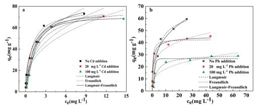
Fig. 8 Adsorption isotherm for the adsorption of (a) Pb( $\mu$ ) and (b) Cd( $\mu$ ) onto BC/FM in a bi-solute system, temperatures = 25 °C; pH = 5; t = 5 h.
