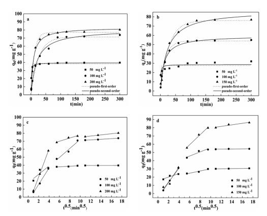
Fig. 6 Pseudo-first-order and pseudo-second-order models for (a) Pb( $_{\parallel}$ ) and (b) Cd( $_{\parallel}$ ) on BC/FM, intraparticle diffusion kinetic model for (c) Pb( $_{\parallel}$ ) and (d) Cd( $_{\parallel}$ ) on the BC/FM; pH = 5; temperature = 298 K; BC/FM dose = 1.25 g L<sup>-1</sup>.
