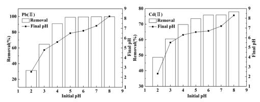
Fig. 5 Effect of pH on adsorption of Pb(II) and Cd(II) on BC/FM. Conditions:  $C_0(Pb(II)) = 100 \text{ mg L}^{-1}$ ,  $C_0(Cd(II)) = 20 \text{ mg L}^{-1}$ , BC/FM dose = 1.25 g L<sup>-1</sup>, temperature = 298 K, and t = 5 h.
