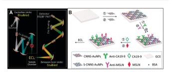
Fig. 12 Scheme of a tabletop spectrofluorometer-potentiostat system for high-resolution ECL spectrum collection, and diagram of the light path (left); general assembly procedure for the wavelength-resolved ECL biosensor for the simultaneous detection of multiple biomarkers (right). 105 Adapted with permission from ref. 105. Copyright 2018 American Chemical Society.
