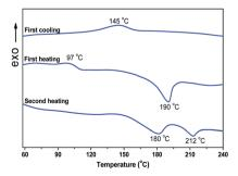
Fig. 3 The DSC curves of DPP-2Py-9 in the first heating, first cooling and second heating processes at 5  $^{\circ}$ C min $^{-1}$  scanning rate under nitrogen flow.
