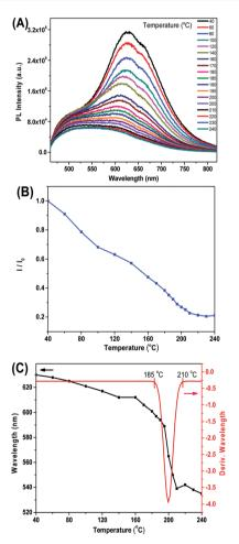
Fig. 7 The temperature-dependent PL changes of **DPP-2Py-9** by the heating process (A), the PL intensity of **DPP-2Py-9** with the variation of temperature (B) and the change of wavelength and differential curve of PL wavelength with the variation of temperature (C).
