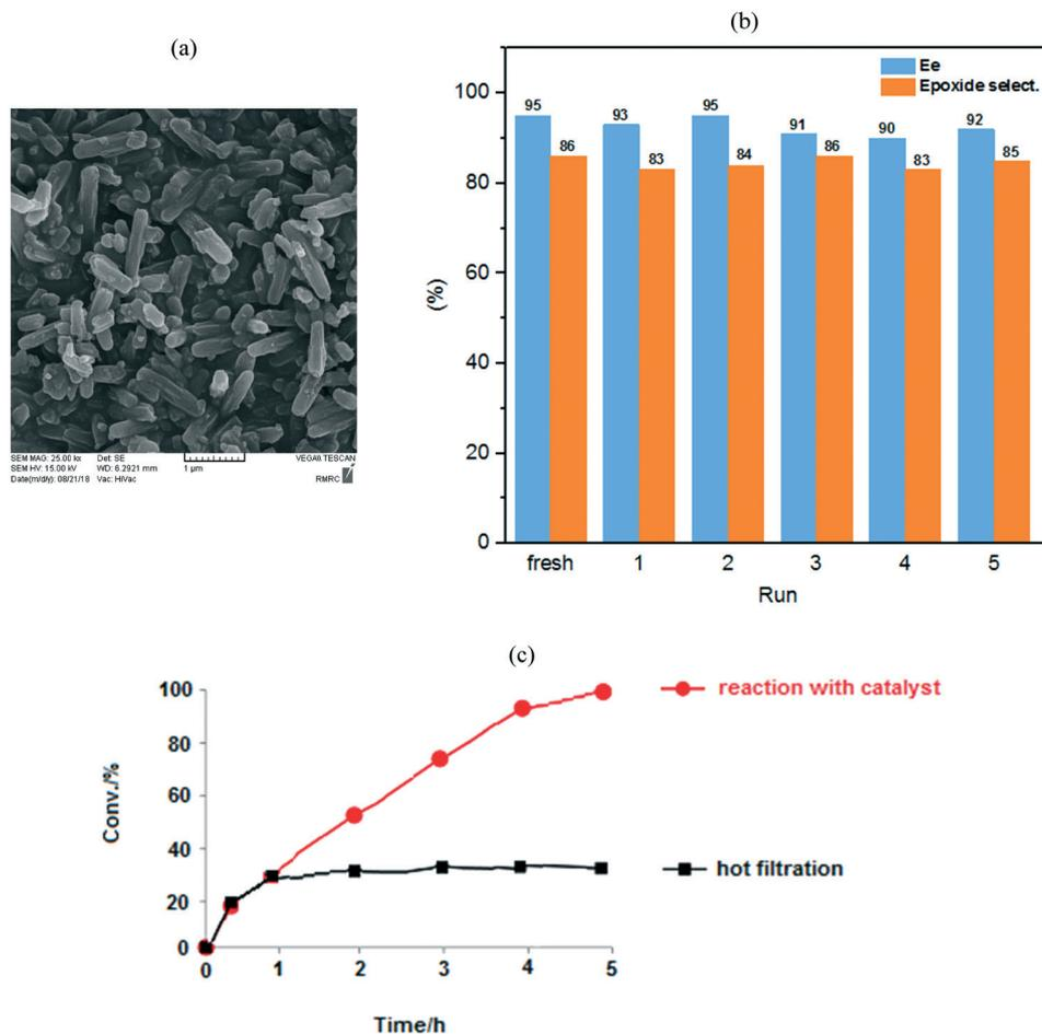
**Fig. 5** (a) The SEM image of the used catalyst in the fifth run. (b) The obtained ee and epoxide selectivity by using the reusable [C-NU-1000-Mo] in the oxidation of styrene to five recycles. (c) Hot filtration test was carried out at 80 °C. The epoxidation of styrene with catalyst (red) and after filtering the catalyst from reaction mixture after 1 h (black).
