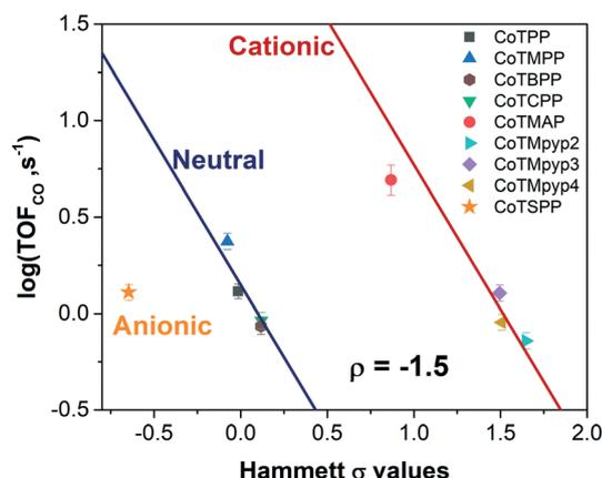
Fig. 4  $\text{TOF}_{\text{CO}}$  of cobalt porphyrin derivatives with various functionalities versus calculated Hammett  $\sigma$  values (potential:  $-0.6 \text{ V}$  vs. RHE, loading:  $8 \times 10^{-10} \text{ mol cm}^{-2}$ ).
