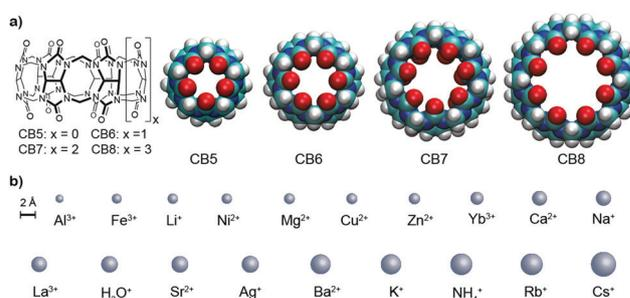
Fig. 1 (a) Chemical structures and their 3D representation (space filling model) of CB*n* and (b) of the metal cations investigated in this study, with sizes drawn to scale with respect to CB*n*; the portal diameters are 2.4 Å for CB5, 3.9 Å for CB6, 5.4 Å for CB7, and 6.9 Å for CB8.
