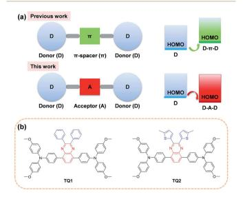
Fig. 1 (a) A schematic illustration of the shift of the HOMO energy level of D $-\pi$ D and D-AD structured organic HTMs. (b) Chemical structures of D-AD structured HTM TQ1 and TQ2 featuring a moderately electron deficient quinoxaline as the core.
