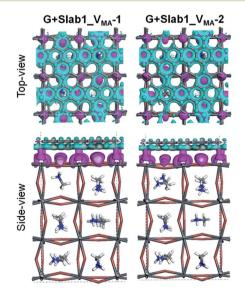
Fig. 19 Electron density difference of the  $V_{MA}$ -containing graphene + MAPbl<sub>3</sub> hybrids (isovalue: 0.003 a.u.). Purple and cyan represent accumulation and depletion of electrons, respectively.
