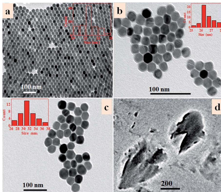
Fig. 1 Transmission electron microscopy (TEM) images of (a) NaYF<sub>4</sub>:Yb,Er (core), (b) NaYF<sub>4</sub>:Yb,Er@NaGdF<sub>4</sub> (UCNP), (c) UCNP–PAA, and (d) PEG–NH<sub>2</sub> modified BPNS (BPNS–NH<sub>2</sub>). The insets in (a–c) indicate the diameter (size) distribution obtained from the count of the corresponding nanoparticles.
