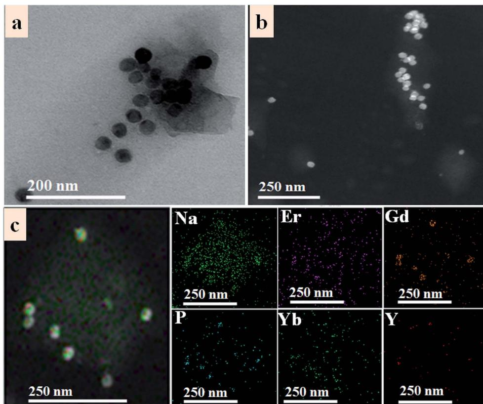
Fig. 2 (a) TEM image of UCNP–BPNS nanocomposite, (b) scanning transmission electron microscope (STEM) image of UCNP–BPNS nanocomposite, and (c) STEM image and the corresponding elemental mapping of UCNP–BPNS nanocomposite.
