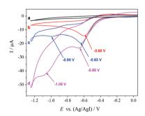
Fig. 1 Cyclic voltammograms recorded on a Pt electrode at 100 mV s<sup>-1</sup> in: (a) DMF containing 0.07 M Bu<sub>4</sub>NPF<sub>6</sub>; (b) solution (a) after addition of 2 mM [(R)-BINAP]Pd(OAc)<sub>2</sub>; (c) solution (b) after addition of 20 mM 1b; (d) solution (c) saturated with CO2
