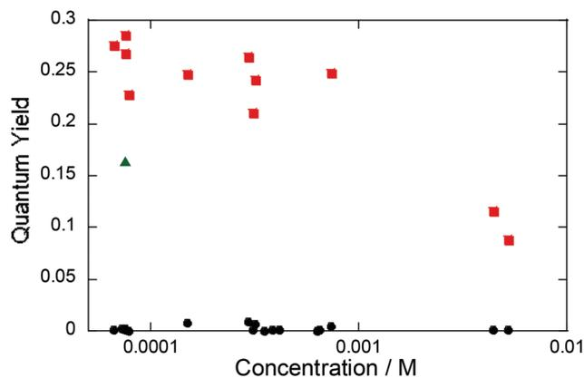
**Fig. 4** Phosphorescence quantum yield of PtCP-fixed glass as a function of PtCP concentration in air (black circle) and under an Ar atmosphere (red square). The green triangle shows that of a PtCP solution in THF with a concentration of 75  $\mu\text{M}$  under an Ar atmosphere.
