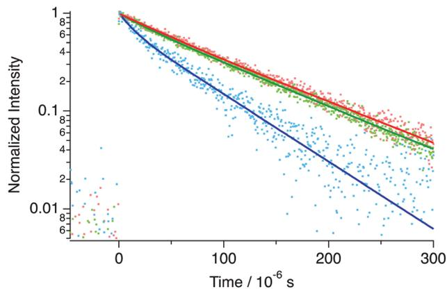
**Fig. 5** Phosphorescence decay of PtCP-fixed glass with different loading concentrations of PtCP: 75  $\mu\text{M}$  (red), 310  $\mu\text{M}$  (green), and 5.1 mM (blue) measured under an Ar-atmosphere with their curve fit (solid lines of the corresponding colors) to single- (75  $\mu\text{M}$ ) and double-exponential (310  $\mu\text{M}$  and 5.1 mM) functions.
