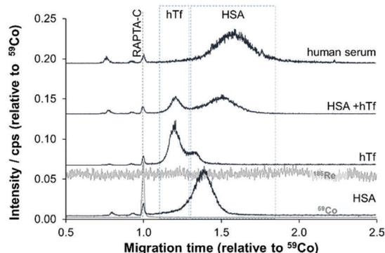
Fig. 3 The CZE-ICP-MS electropherograms for reaction mixtures of RAPTA-C with HSA, hTf and HSA/hTf (50  $\mu\text{M}$ , 1:1) in saline solution and human serum after 96 h incubation, using PVP-coated capillaries.  $[\text{Co}(\text{acac})_3]$  was added as an internal standard and used as the EOF marker.
