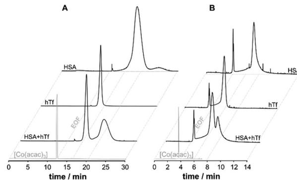
Fig. 2 The CE-UV (214 nm) electropherograms of  $[\text{Co}(\text{acac})_3]$  (10  $\mu\text{M}$ , internal standard, EOF marker) and the serum proteins (100  $\mu\text{M}$ ) HSA and hTf and a HSA/hTf mixture (1:1) using either (A) PVP- or (B) PB-coated capillaries.
