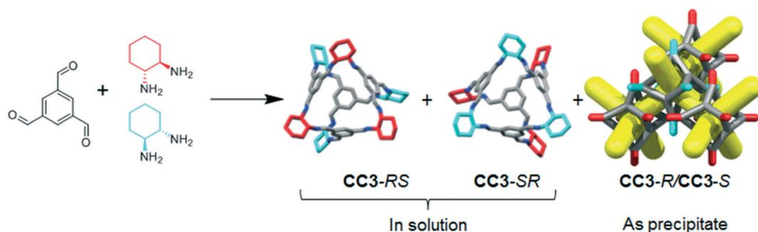
**Fig. 2** TFB and *rac*-CHDA react to form CC3-*RS* and CC3-*SR*, which are soluble and remain in solution, as well as CC3-*R* and CC3-*S*, which immediately co-crystallise to form the racemate, CC3-*R*/CC3-*S*, as a white precipitate. Colours as in Fig. 1.
