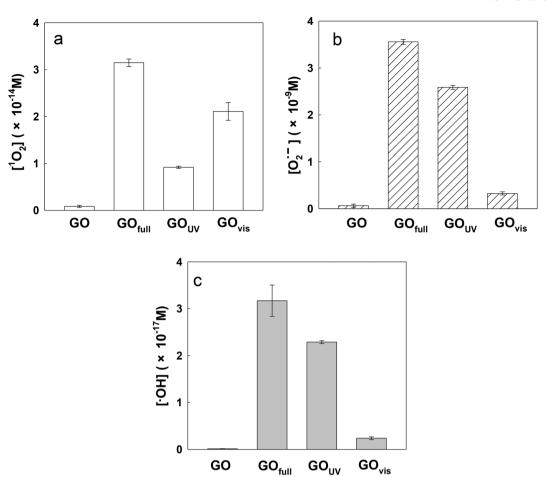
Fig. 3 Steady-state concentrations of (a) singlet oxygen ( $^{1}O_{2}$ ), (b) hydroxyl radicals ('OH), and (c) superoxide radical anions ( $O_{2}$ ) in GO suspensions in the dark (GO) and exposed to full-spectrum solar (GO<sub>full</sub>), UV (GO<sub>UV</sub>), and visible light (GO<sub>vis</sub>). [GO] = 10 mg L<sup>-1</sup>; pH = 7.
