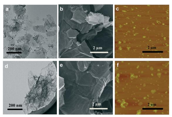
Fig. 5 TEM micrographs, SEM micrographs and AFM images of GO exposed to UV light ( $\lambda$  = 290–420 nm) (a–c) and exposed to UV light with t-BuOH (d–f).
