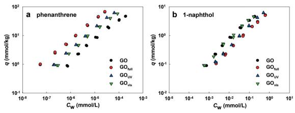
Fig. 7 Isotherms of adsorption of phenanthrene (a) and 1-naphthol (b) onto the colloidal GO,  $GO_{full}$ ,  $GO_{UV}$  and  $GO_{vis}$  suspensions; q (mmol  $kg^{-1}$ ) and  $C_W$  (mmol  $L^{-1}$ ) are the equilibrium concentrations of an adsorbate on GO and in the solution, respectively.
