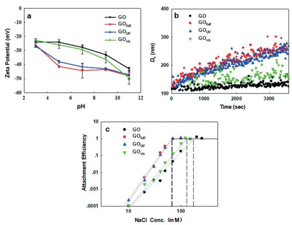
Fig. 6 Influence of different irradiation types on the physicochemical properties of graphene oxide in water. (a) Zeta potential; (b) agglomeration kinetics.  $[Na^+] = 30 \text{ mg L}^{-1}$ , pH = 7; (c) attachment efficiency as a function of NaCl concentration at pH 7.
