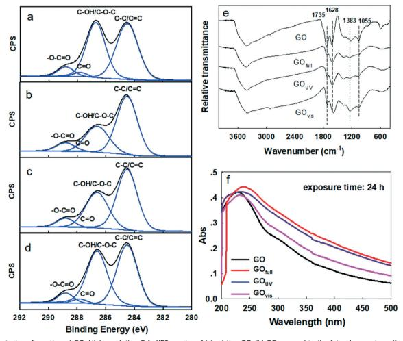
Fig. 1 Photo-transformation of GO. High resolution C 1s XPS spectra of (a) pristing GO, (b) GO exposed to the full solar spectrum ( $\lambda > 290$  nm), (c) GO exposed to UV light ( $\lambda$  = 290–420 nm), and (d) GO exposed to visible light ( $\lambda$  > 420 nm). Changes in GO after exposure to light of different wavelengths were also determined via (e) FTIR spectroscopy and (f) UV-vis absorbance spectroscopy.
