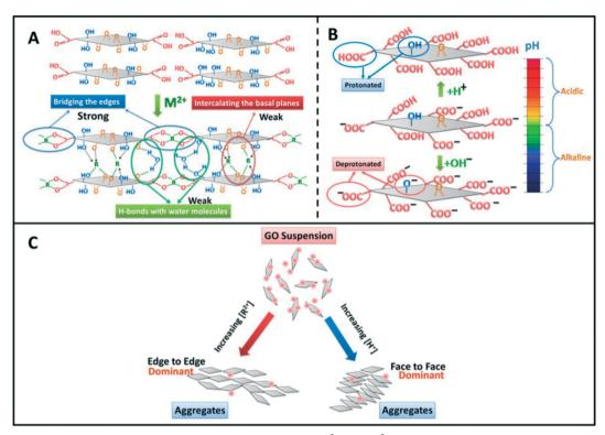
Fig. 8 GO aggregation mechanisms: (A) cross-linking by divalent cations (Mg<sup>2+</sup> and Ca<sup>2+</sup>), (B) deprotonation of the carboxyl groups at the edges when pH increases, and (C) summary of aggregation modes of GO nanosheets. 64 Reprinted with permission from ref. 64. Copyright 2013, American Chemical Society.
