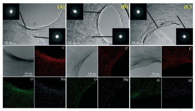
Fig. 9 TEM, selected area electron diffraction (SAED) and element mapping pattern of GO aggregates in the presence of Na<sup>+</sup> (A), Mg<sup>2+</sup> (B) or Al<sup>3+</sup> (C) electrolyte (Na<sup>+</sup>: 50 mM, Mg<sup>2+</sup>: 1 mM, Al<sup>3+</sup>: 0.1 mM and GO: 20 mg L<sup>-1</sup>). Reprinted with permission from ref. 67. Copyright 2017, Elsevier.
